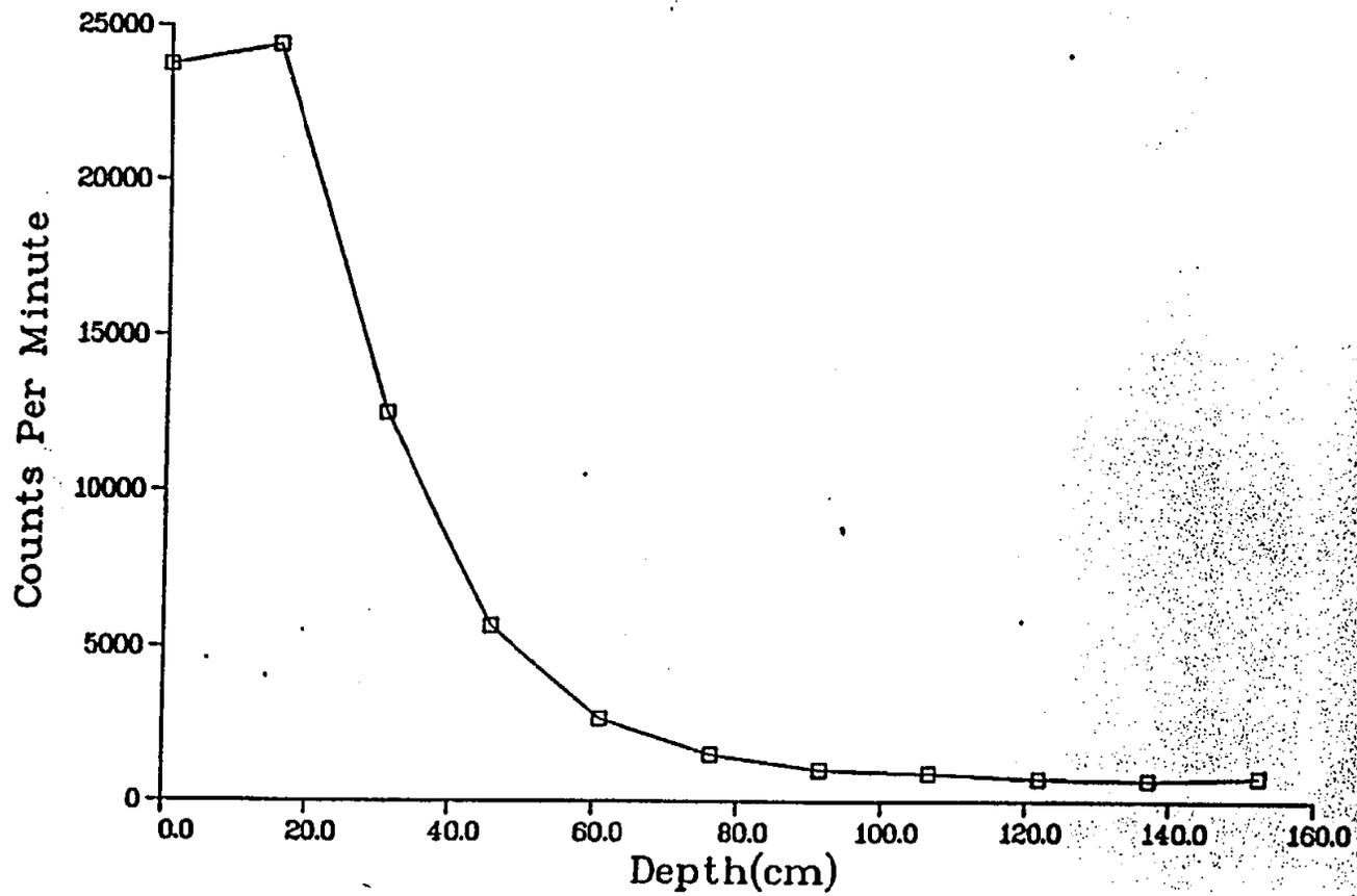
Fig. II-3. Gamma profile of core hole MJC21 (see Fig. 6)
