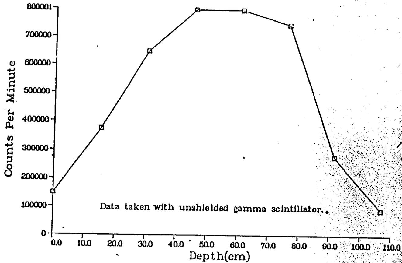
Fig. II-14. Gamma profile of core hole MJC32 (see Fig. 8)
