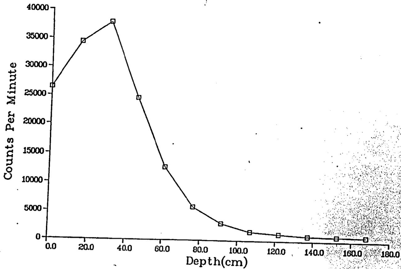
Fig. II-7. Gamma profile of core hole MJC25 (see Fig. 6)
