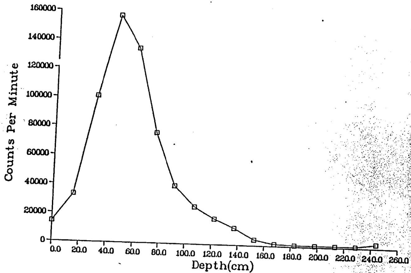
Fig. II-16. Gamma profile of core hole MJC44 (see Fig. 6)
