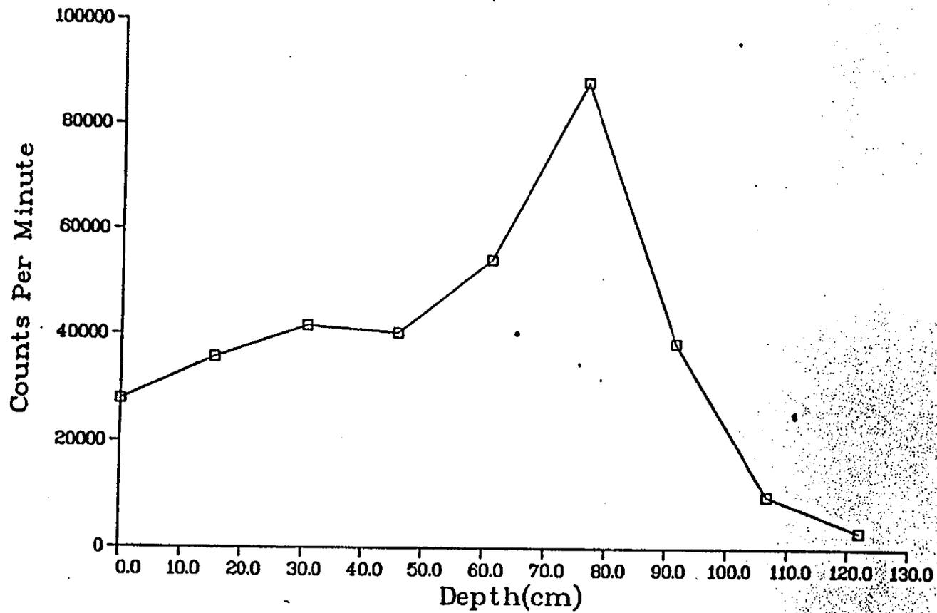
Fig. II-9. Gamma profile of core hole MJC27 (see Fig. 6)
