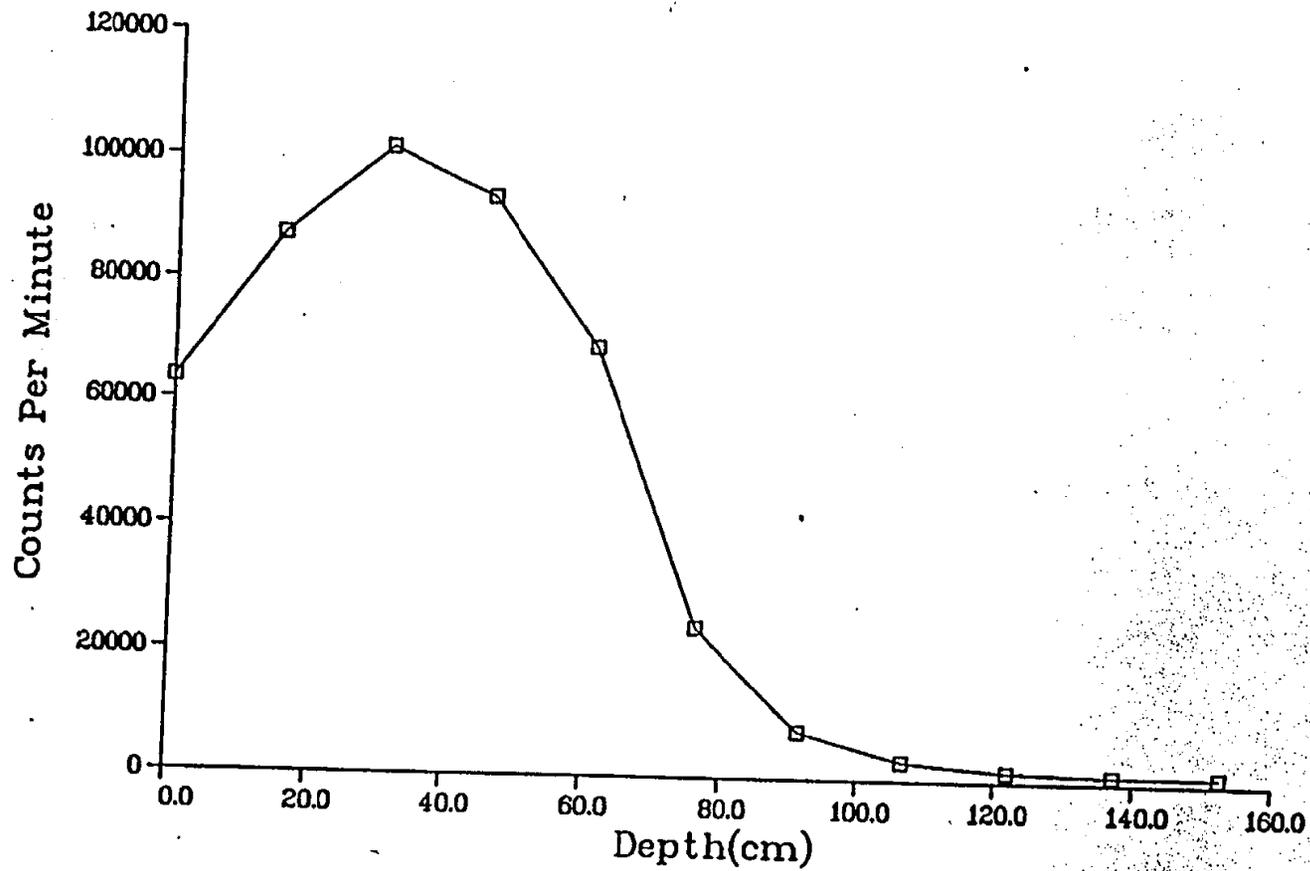
Fig. II-5. Gamma profile of core hole MJC23 (see Fig. 6)
