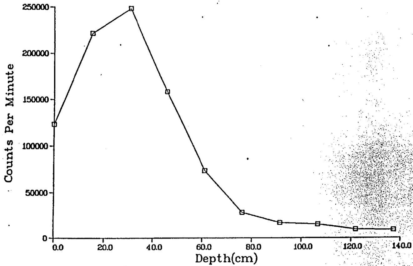
Fig. II-17. Gamma profile of core hole MJC45 (see Fig. 6)
