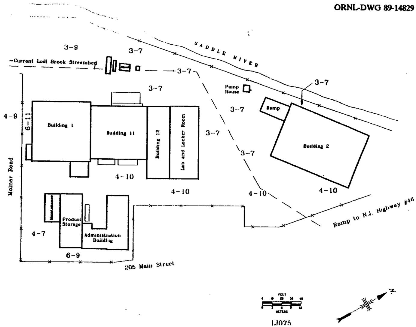
Fig. 1. Gamma radiation levels ( $\mu\text{R/h}$ ) measured on the surface at 205 Main Street, Lodi, New Jersey (LJ075).
