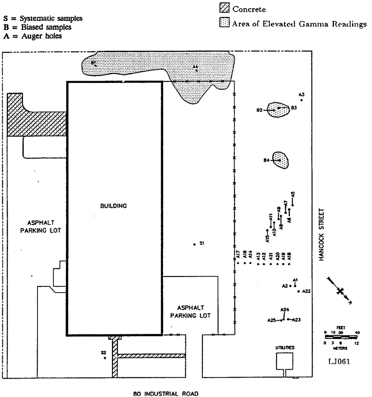
Fig. 2. Diagram showing locations of soil samples taken at 80 Industrial Road, Lodi, New Jersey (LJ061).
