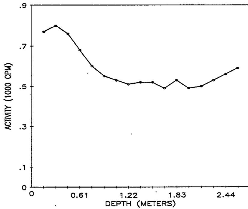
Fig. 6. Gamma profile for auger hole 5 (LJ061A5) at 80 Industrial Road, Lodi, New Jersey.
