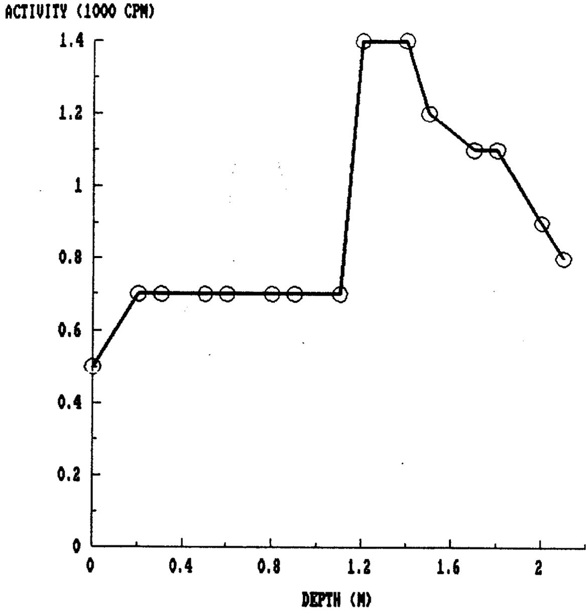
Fig. 4. Gamma profile for auger hole 2 (LJ028A2) at 9 Hancock Street, Lodi, New Jersey.
