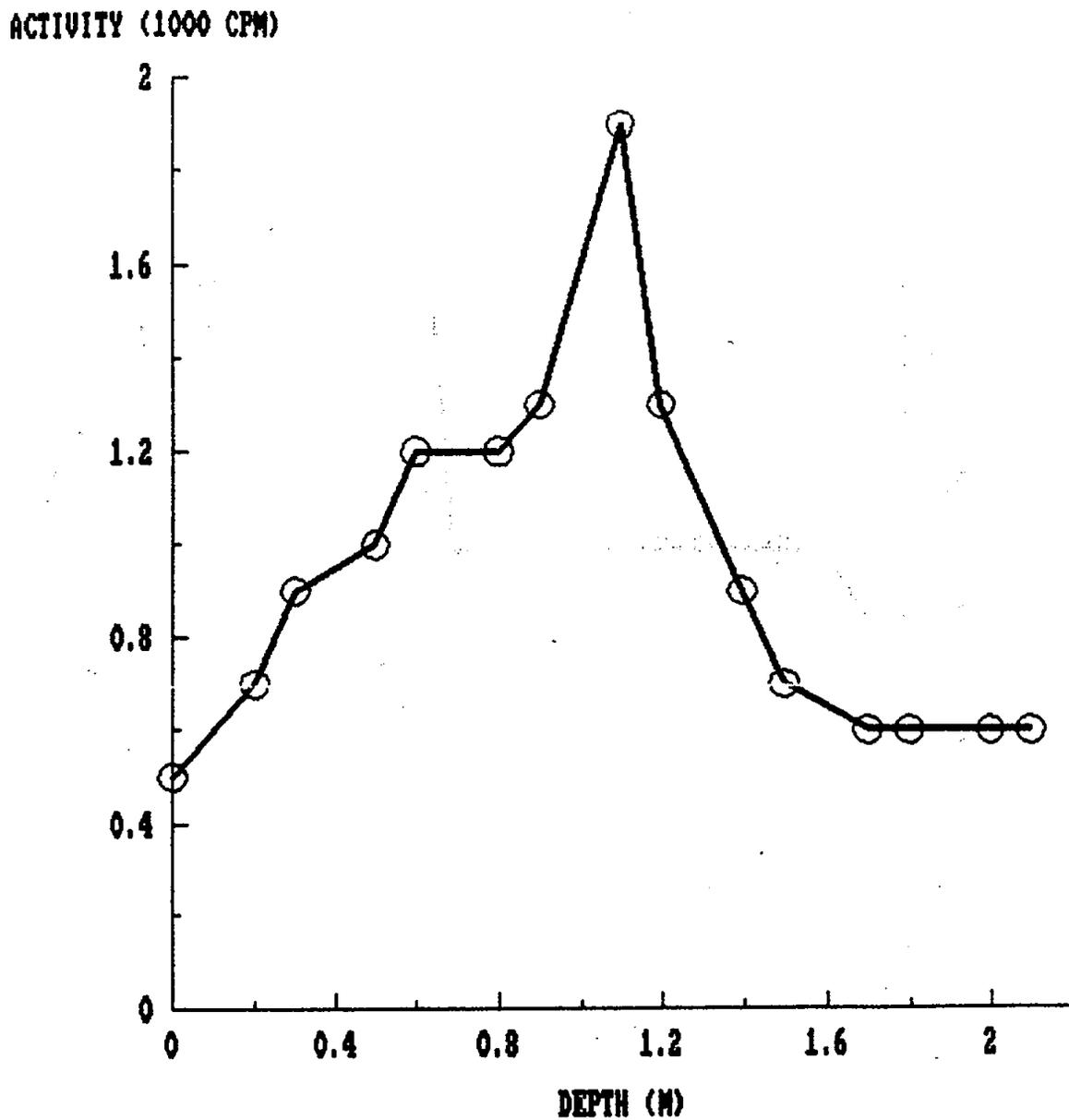
Fig. 3. Gamma profile for auger hole 1 (LJ028A1) at 9 Hancock Street, Lodi, New Jersey.
