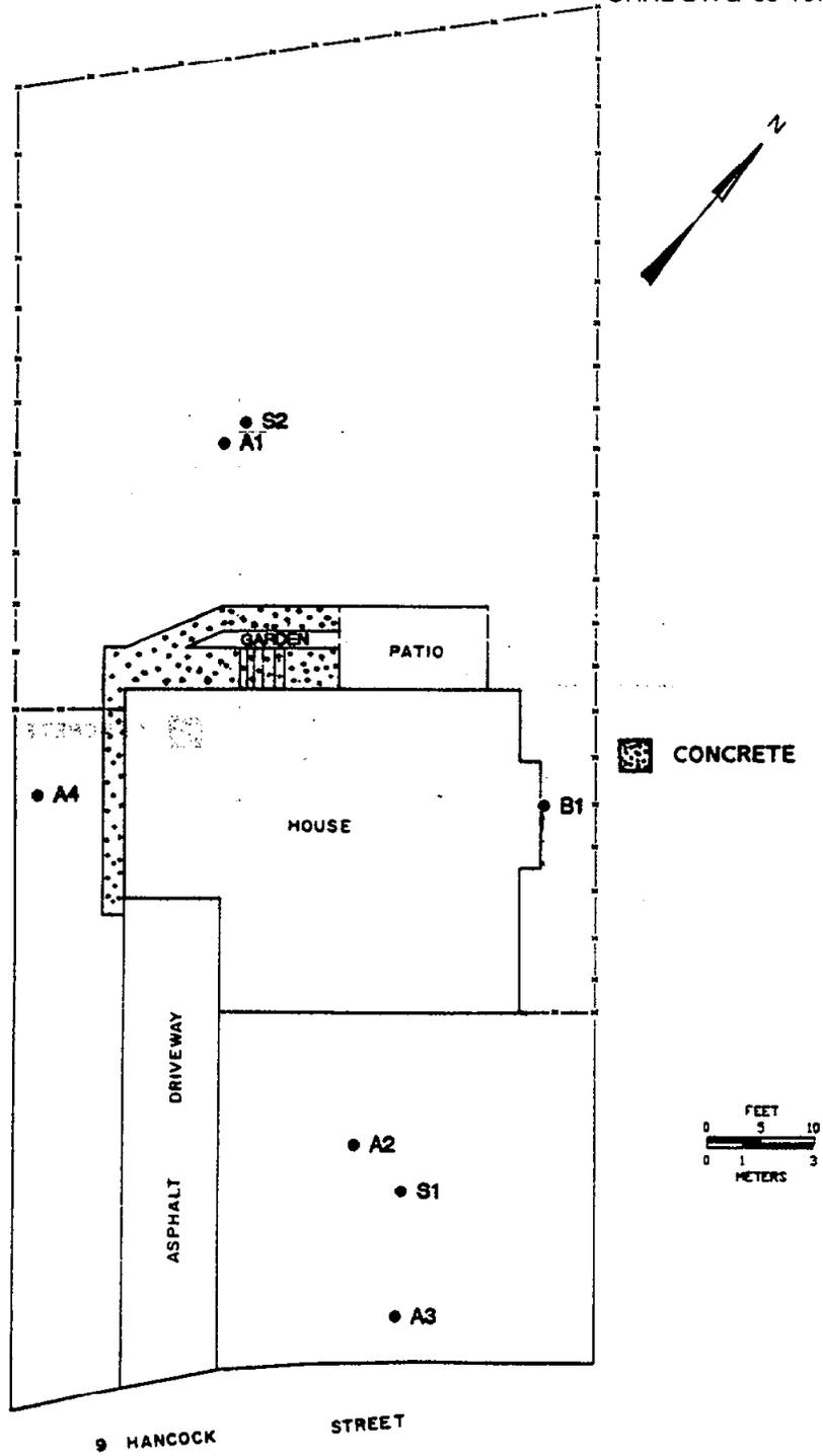
Fig. 2. Diagram showing locations of soil samples taken at 9 Hancock Street, Lodi, New Jersey (LJ028).
