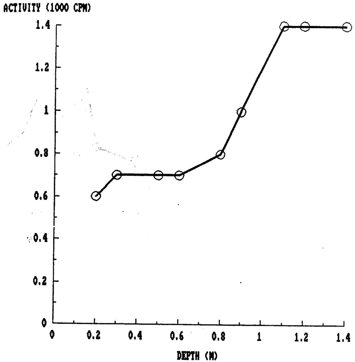
Fig. 5. Gamma profile for auger hole 3 (LJ028A3) at 9 Hancock Street, Lodi, New Jersey.
