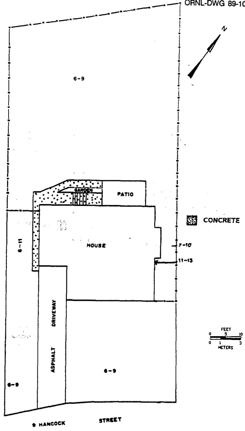
Fig. 1. Gamma radiation levels ( $\mu\text{R/h}$ ) measured on the surface at 9 Hancock Street, Lodi, New Jersey (LJ028).
