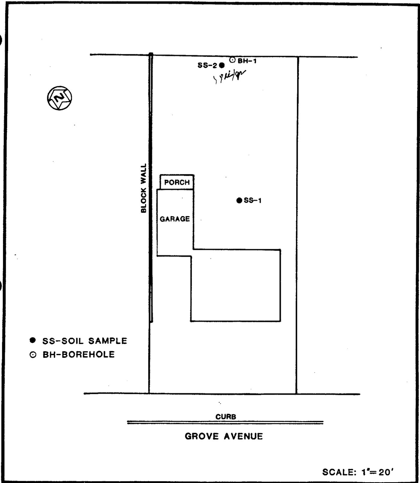
FIGURE 4-11 LOCATIONS OF SURFACE SOIL SAMPLES AND BOREHOLE AT 38 GROVE AVENUE
