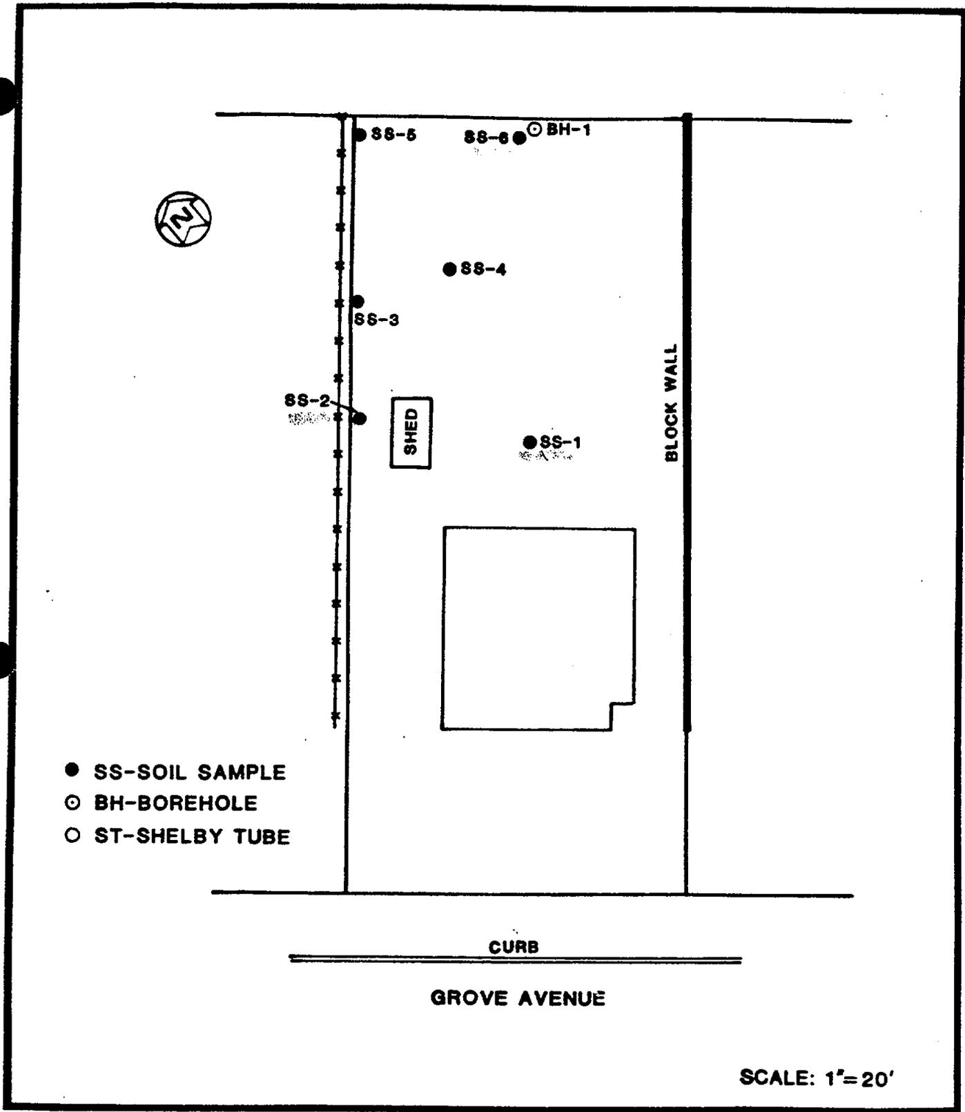
FIGURE 4-10B LOCATIONS OF SURFACE SOIL SAMPLES AND BOREHOLE AT 34 GROVE AVENUE
