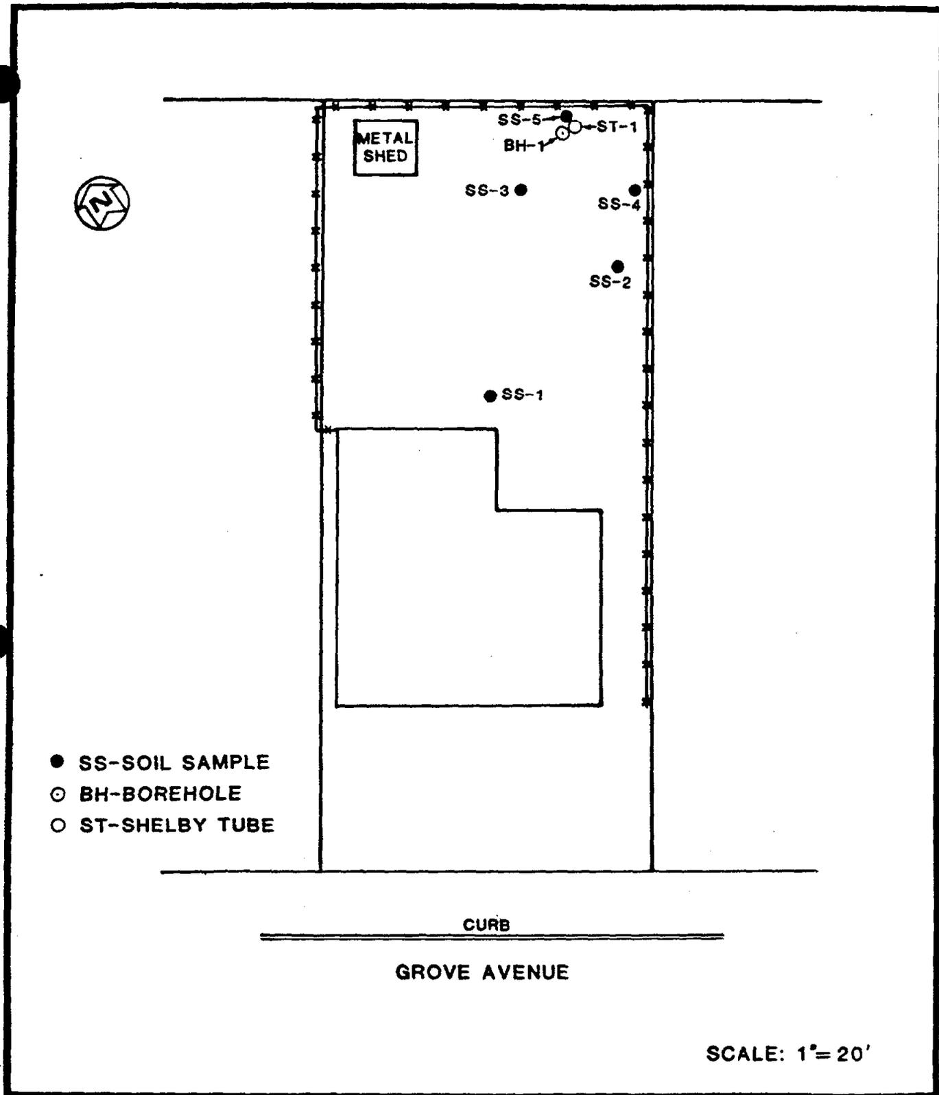
FIGURE 4-7B LOCATIONS OF SURFACE SOIL SAMPLES, BOREHOLE, AND SHELBY TUBE CORE SAMPLE AT 22 GROVE AVENUE
