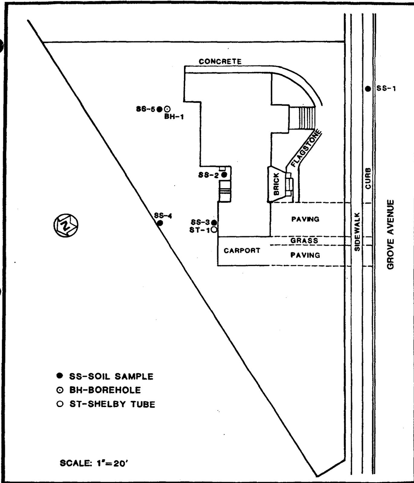
FIGURE 4-4B LOCATIONS OF SURFACE SOIL SAMPLES, BOREHOLE, AND SHELBY TUBE CORE SAMPLE AT 10 GROVE AVENUE
