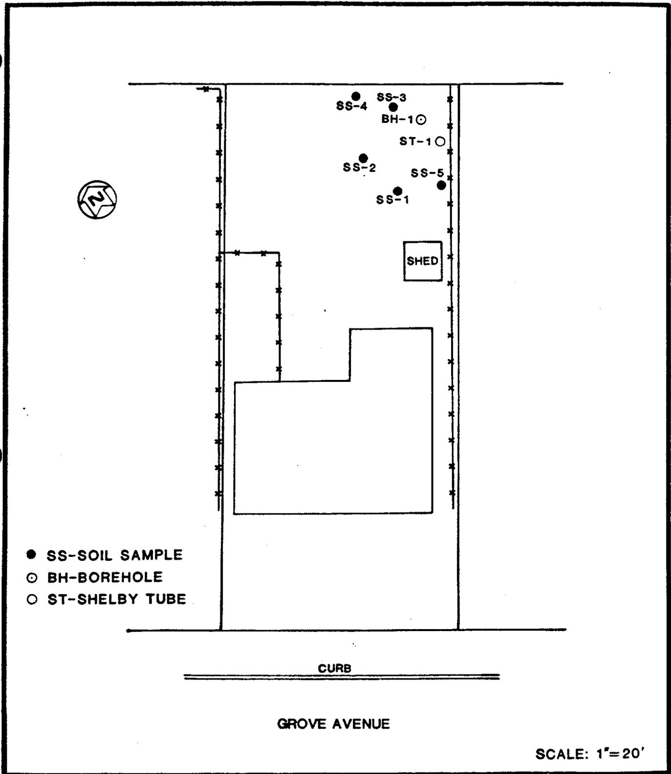
FIGURE 4-8B LOCATIONS OF SURFACE SOIL SAMPLES, BOREHOLE, AND SHELBY TUBE CORE SAMPLE AT 26 GROVE AVENUE
