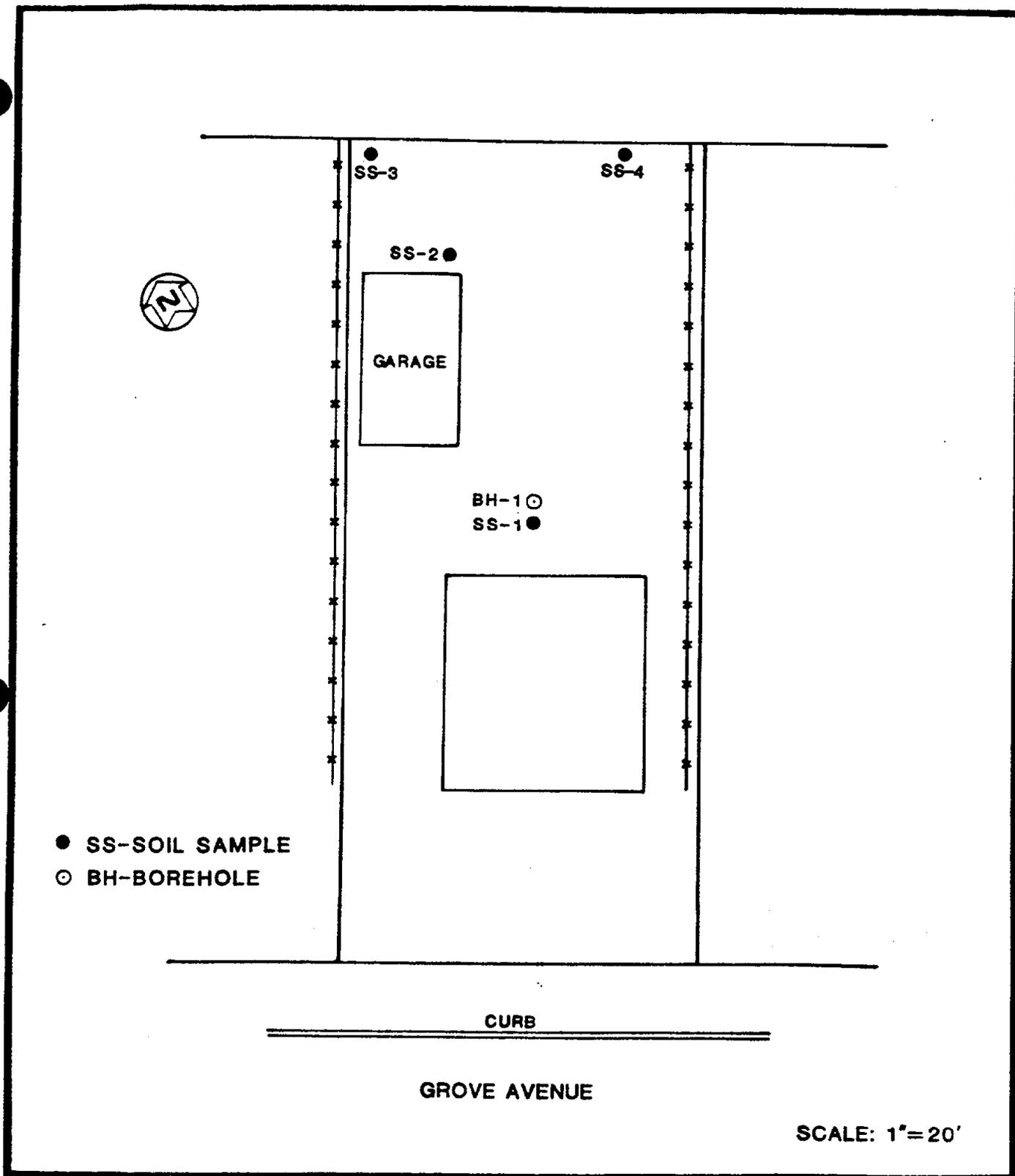
FIGURE 4-9B LOCATIONS OF SURFACE SOIL SAMPLES AND BOREHOLE AT 30 GROVE AVENUE
