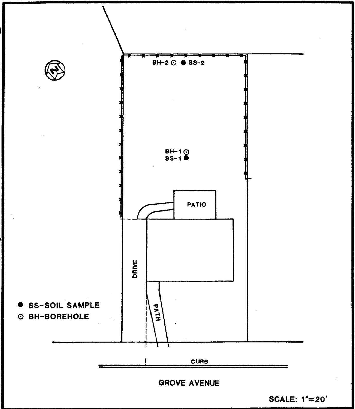
FIGURE 4-6 LOCATIONS OF SURFACE SOIL SAMPLES AND BOREHOLES AT 18 GROVE AVENUE
