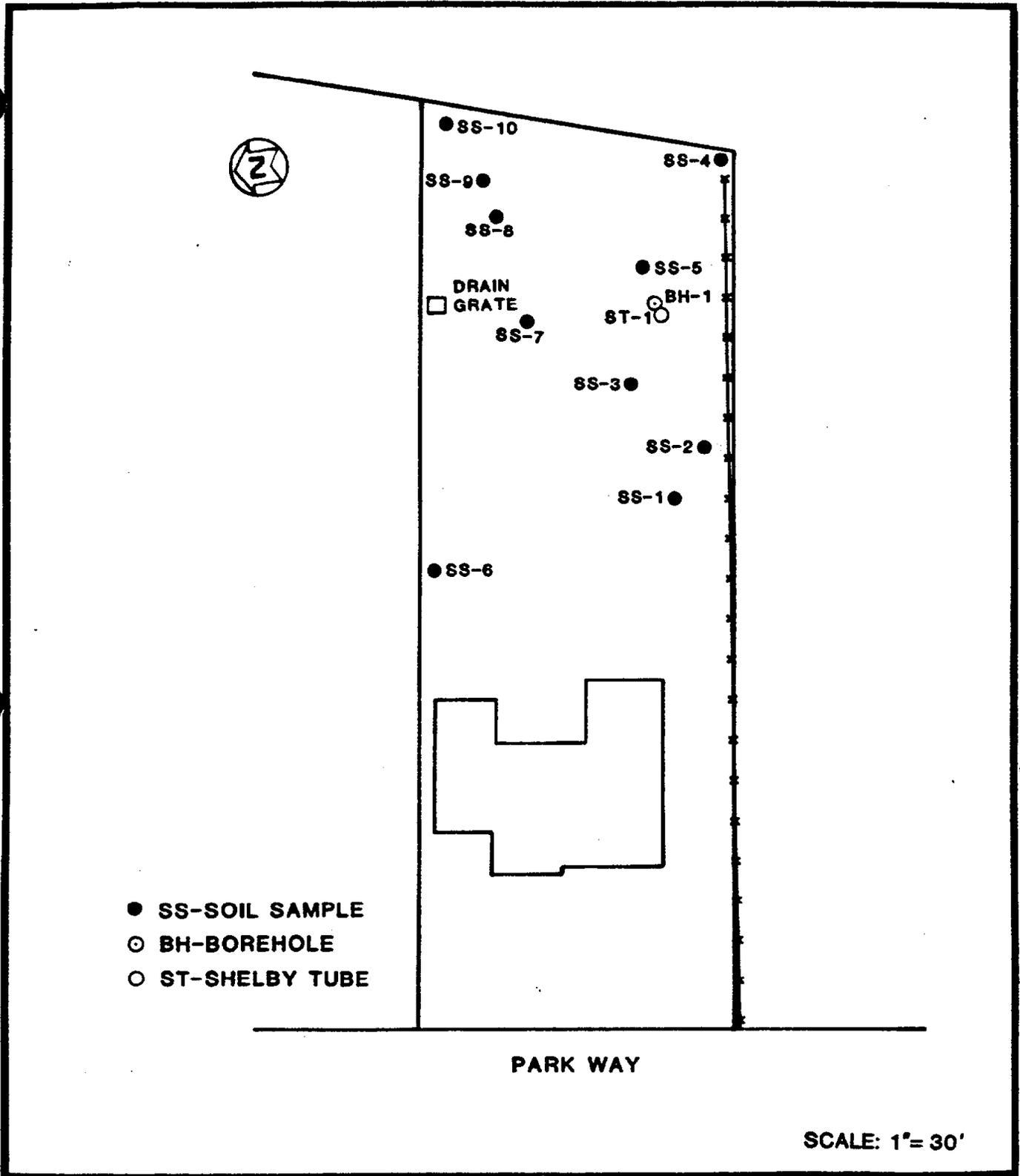
FIGURE 4-3B LOCATIONS OF SURFACE SOIL SAMPLES, BOREHOLE, AND SHELBY TUBE CORE SAMPLE AT 90 PARK WAY
