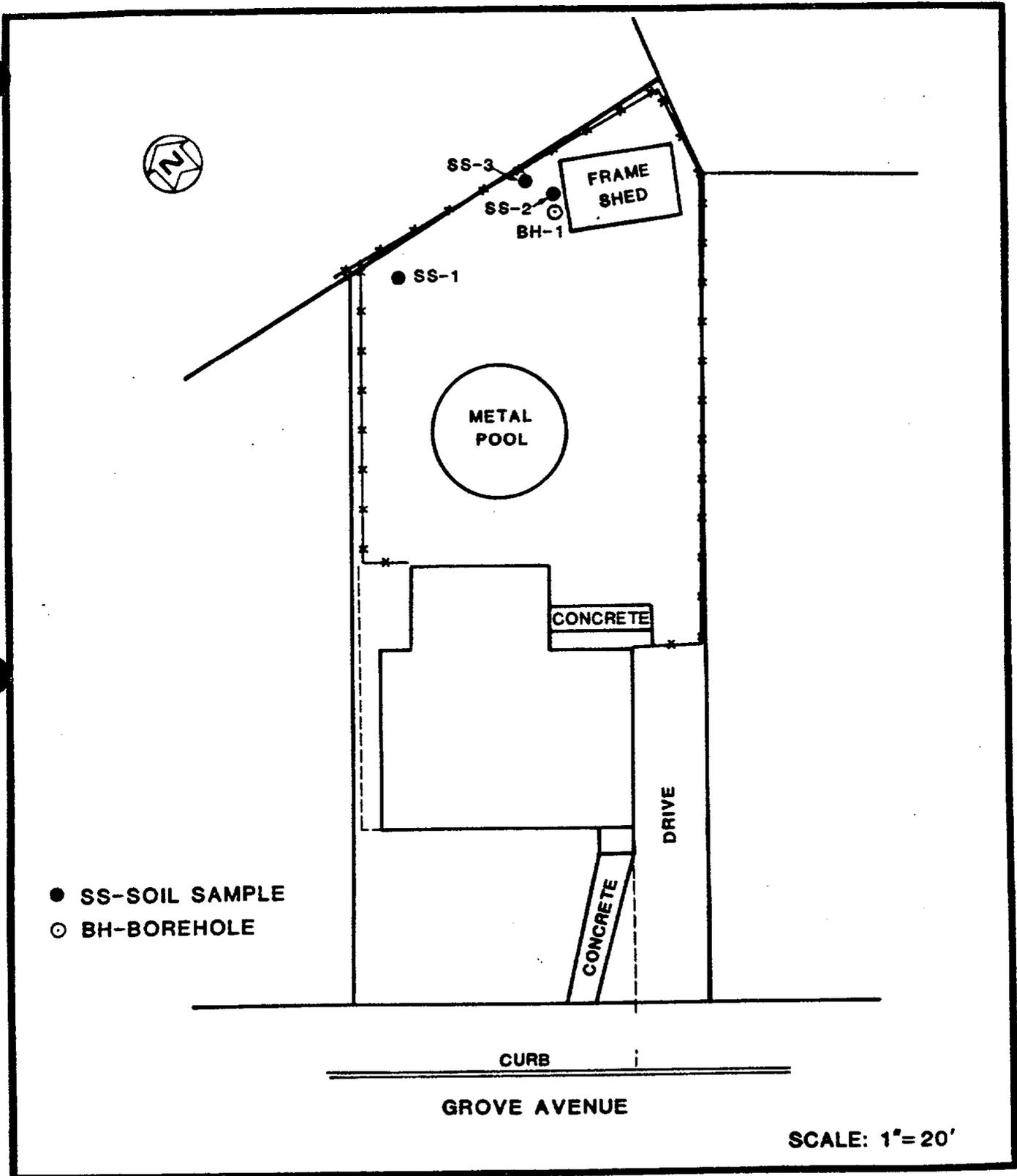
FIGURE 4-5 LOCATIONS OF SURFACE SOIL SAMPLES AND BOREHOLE AT 14 GROVE AVENUE
