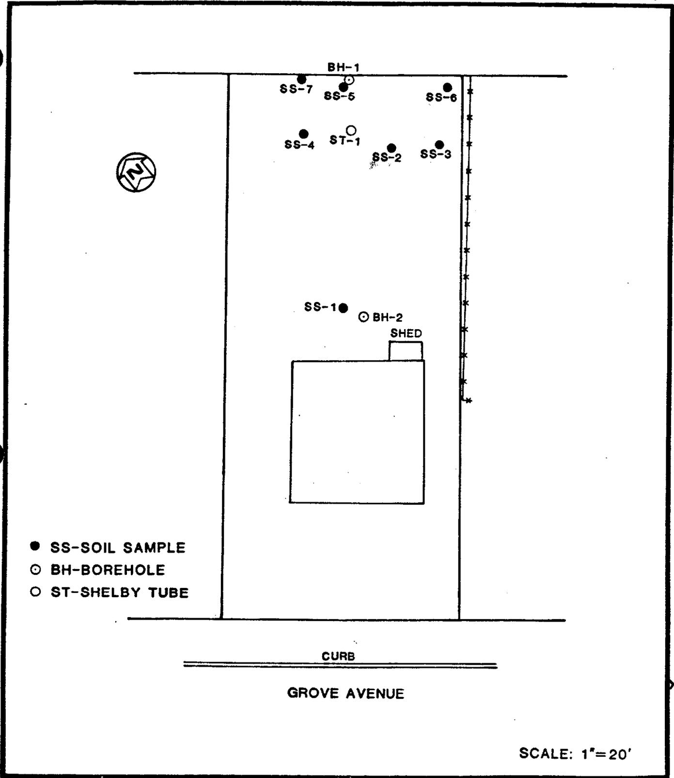
FIGURE 4-12B LOCATIONS OF SURFACE SOIL SAMPLES, BOREHOLES, AND SHELBY TUBE CORE SAMPLE AT 42 GROVE AVENUE
