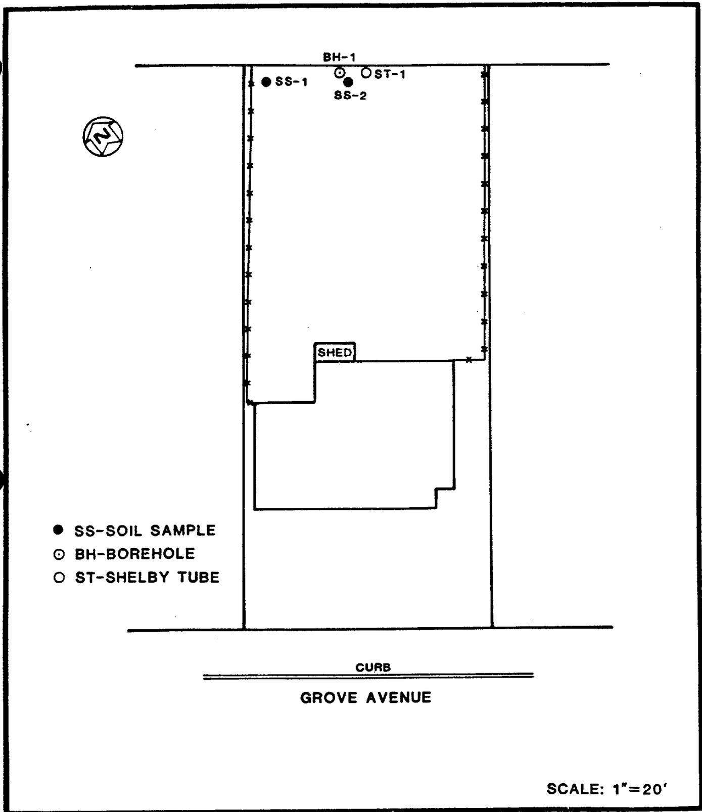
FIGURE 4-13 LOCATIONS OF SURFACE SOIL SAMPLES, BOREHOLE, AND SHELBY TUBE CORE SAMPLE AT 46 GROVE AVENUE
