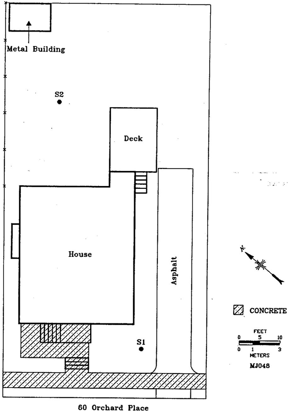
Fig. 2. Diagram showing locations of soil samples taken at 60 Orchard Place, Maywood, New Jersey (MJ048).
