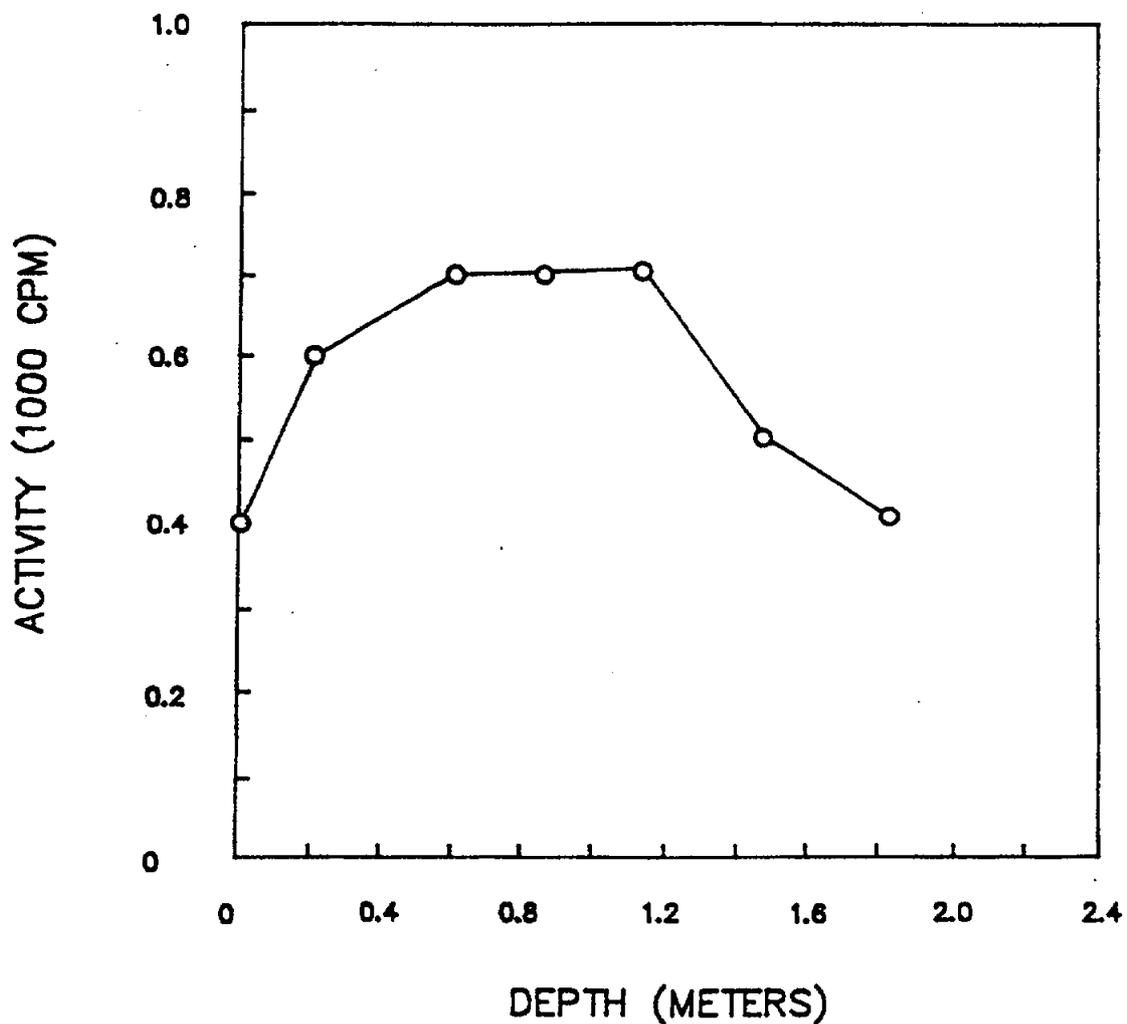
Fig. 5. Gamma profile for auger hole 3 (LJ045A3) at 30 Long Valley Road, Lodi, New Jersey.
