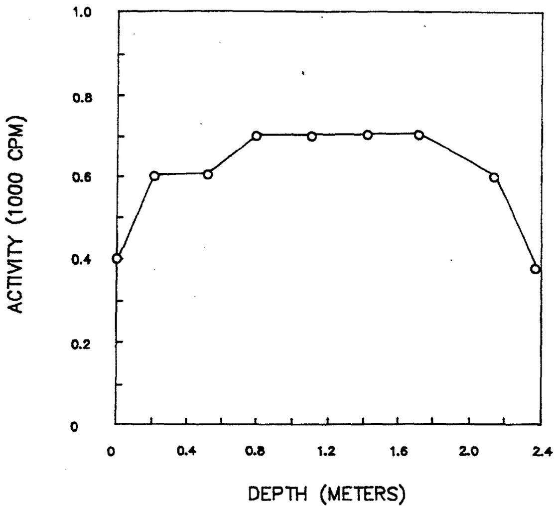
Fig. 6. Gamma profile for auger hole 4 (LJ045A4) at 30 Long Valley Road, Lodi, New Jersey.
