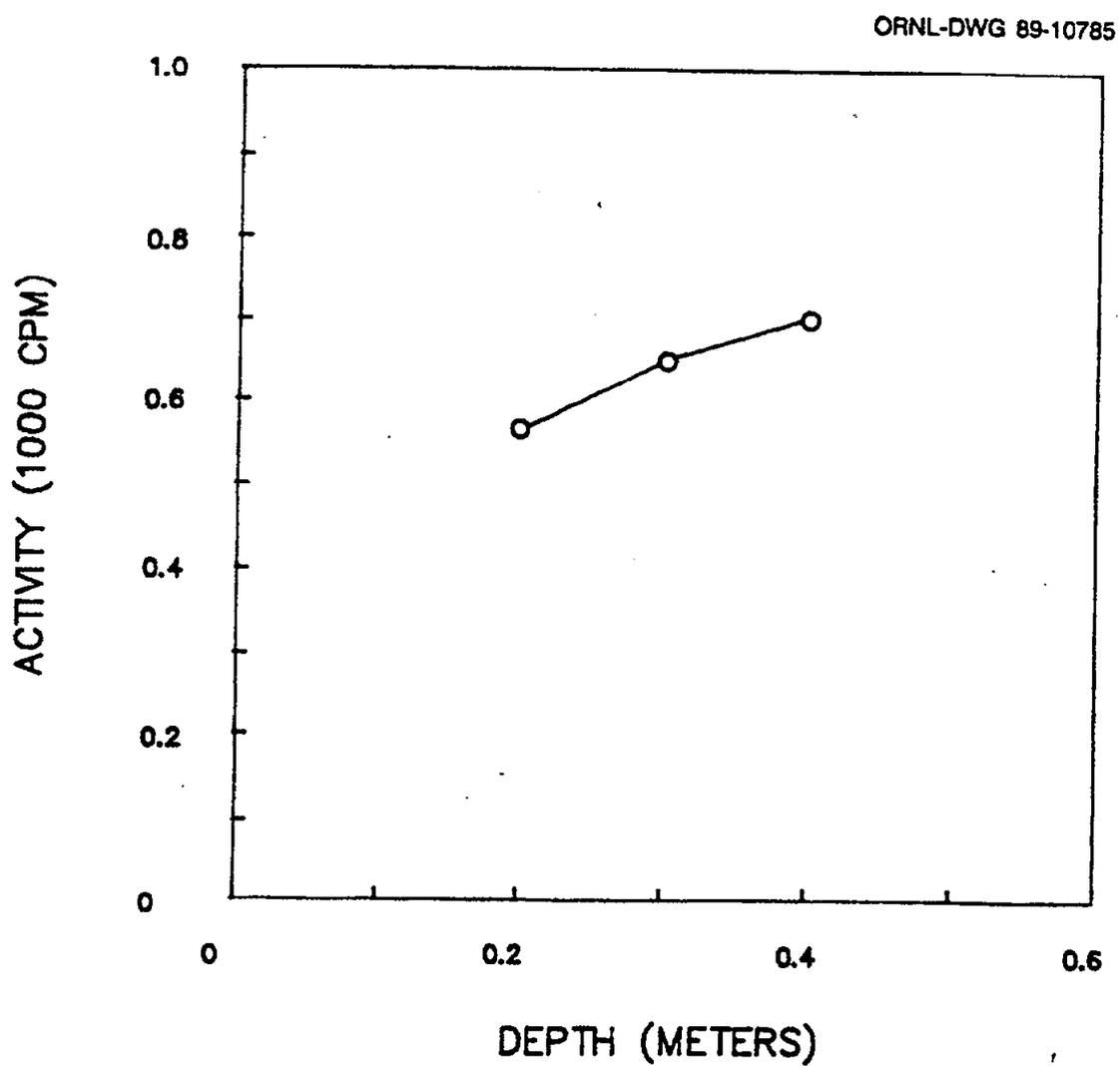
Fig. 8. Gamma profile for auger hole 7 (LJ045A7) at 30 Long Valley Road, Lodi, New Jersey.
