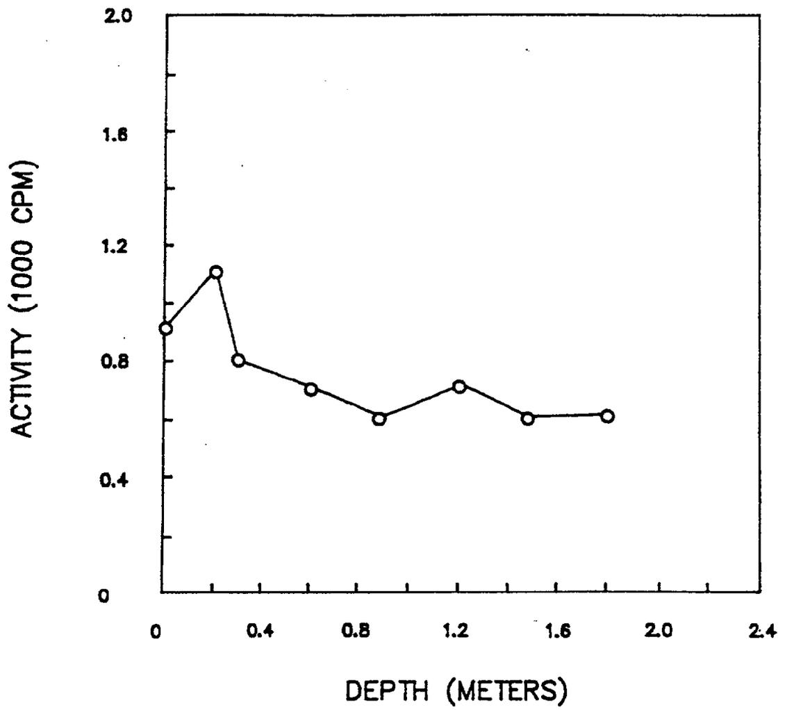
Fig. 3. Gamma profile for auger hole 1 (LJ045A1) at 30 Long Valley Road, Lodi, New Jersey.
