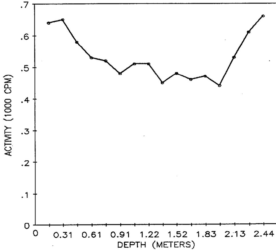
Fig. 3. Gamma profile for auger hole 1 (LJ068A1) at 112 Columbia Lane, Lodi, New Jersey.
