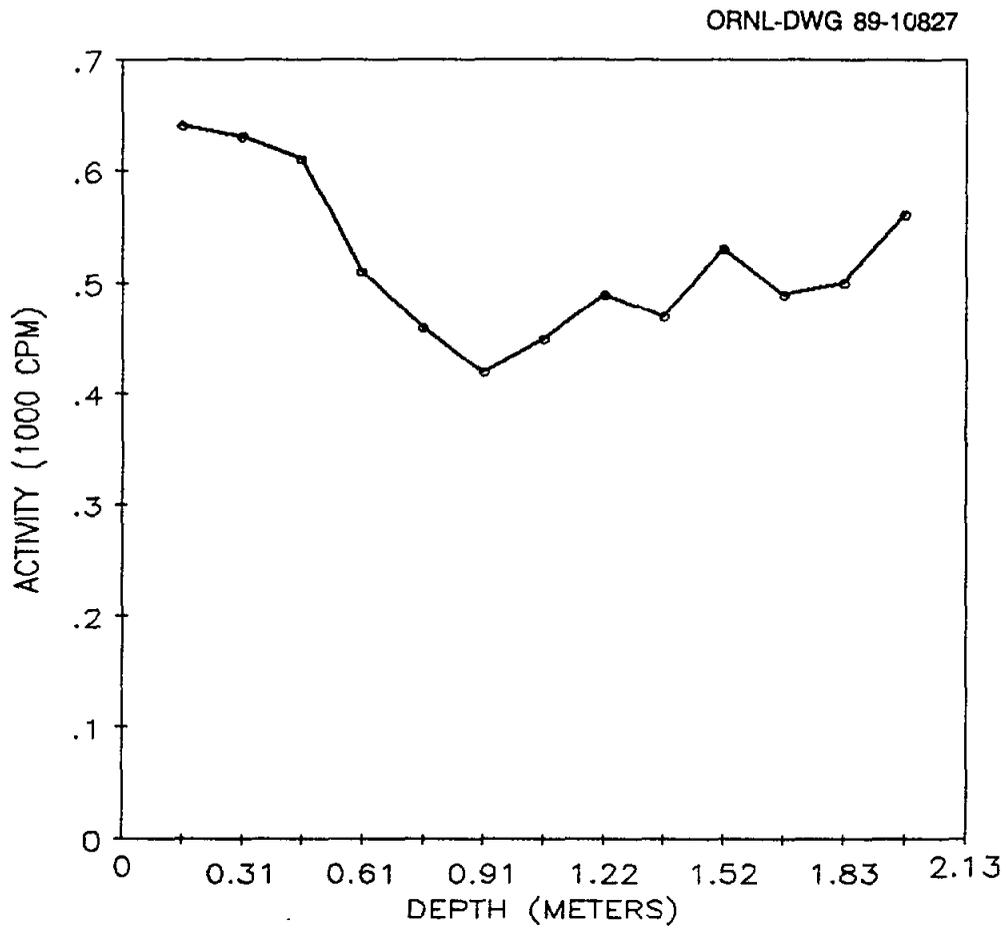
Fig. 4. Gamma profile for auger hole 2 (LJ068A2) at 112 Columbia Lane, Lodi, New Jersey.
