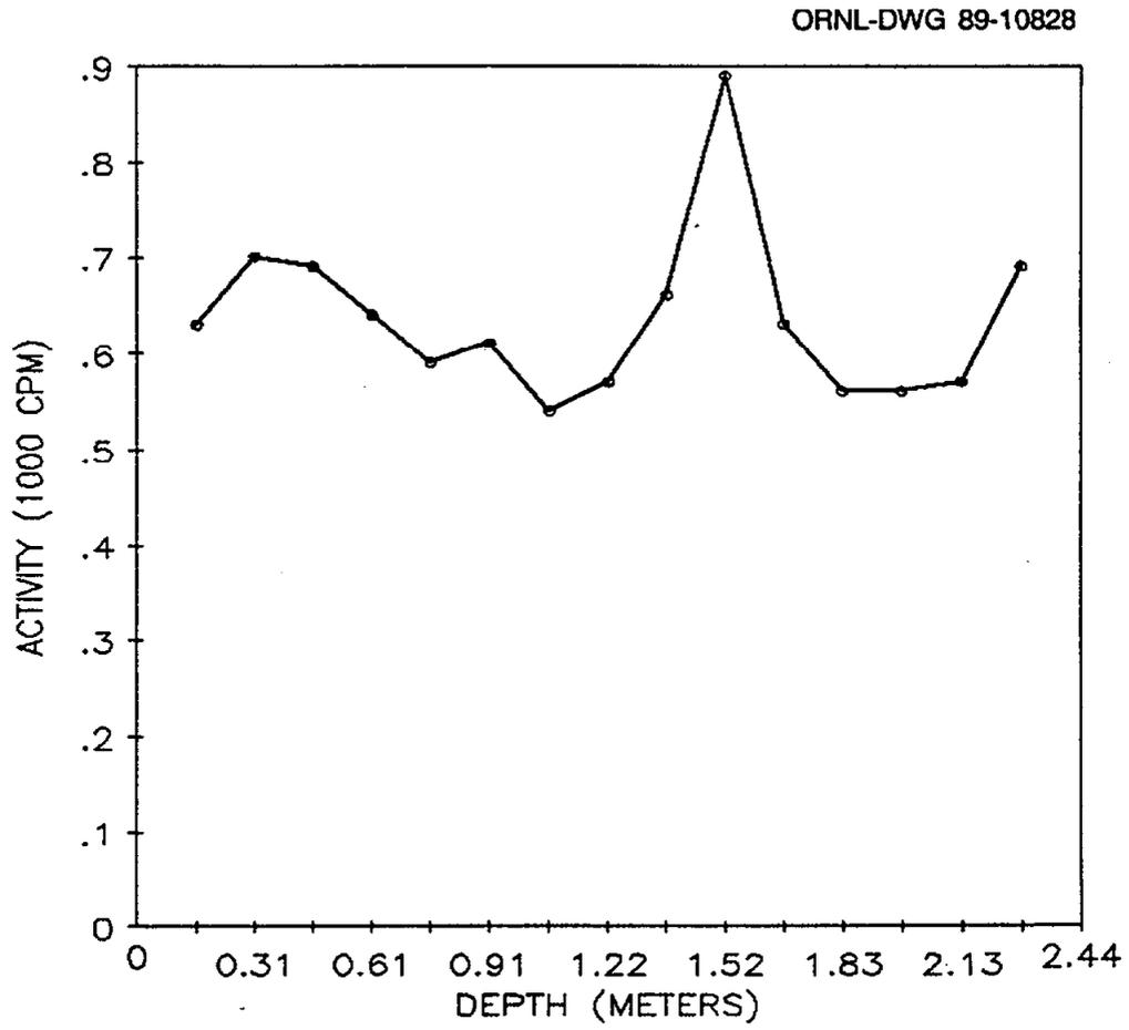
Fig. 5. Gamma profile for auger hole 3 (LJ068A3) at 112 Columbia Lane, Lodi, New Jersey.
