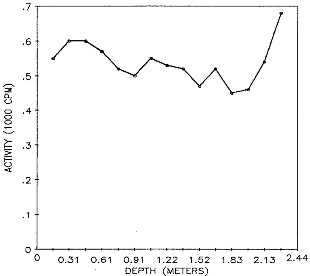
Fig. 6. Gamma profile for auger hole 4 (LJ068A4) at 112 Columbia Lane, Lodi, New Jersey.
