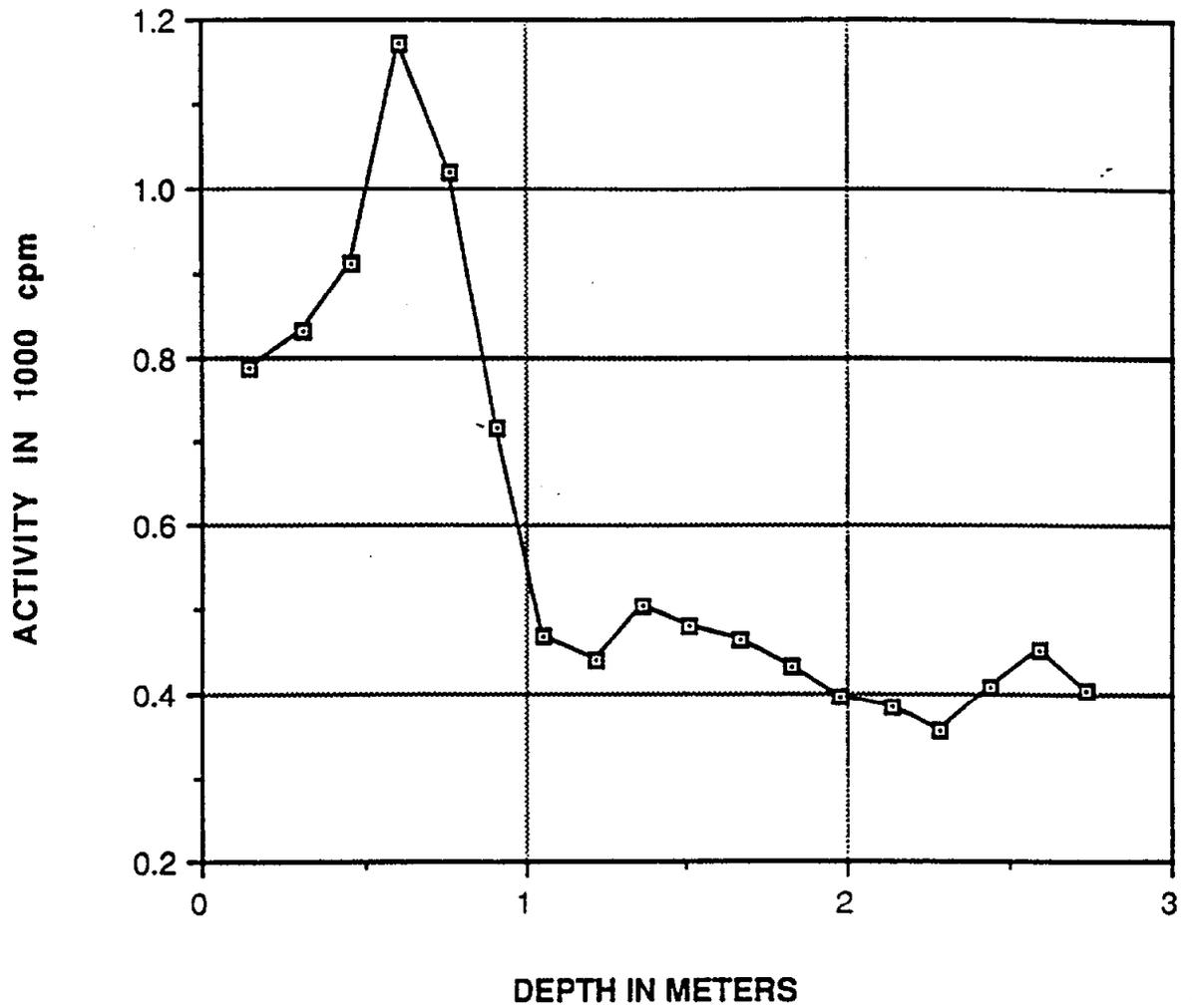
Fig. 6. Gamma profile for auger hole 5 (MJ041A5) at 142 West Central Avenue, Maywood, New Jersey.
