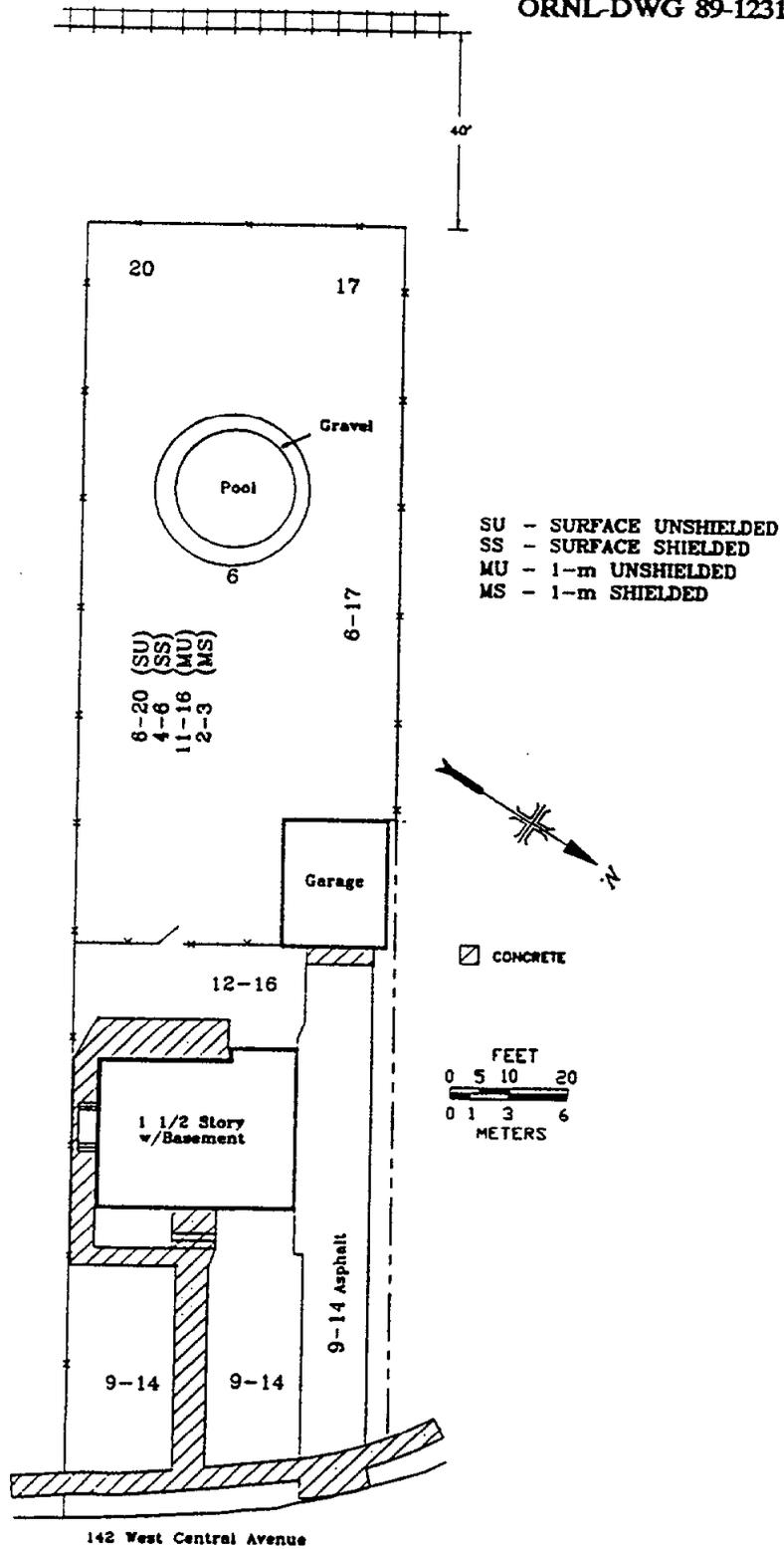
Fig. 1. Gamma radiation levels ( $\mu\text{R/h}$ ) measured on the surface at 142 West Central Avenue, Maywood, New Jersey (MJ041).
