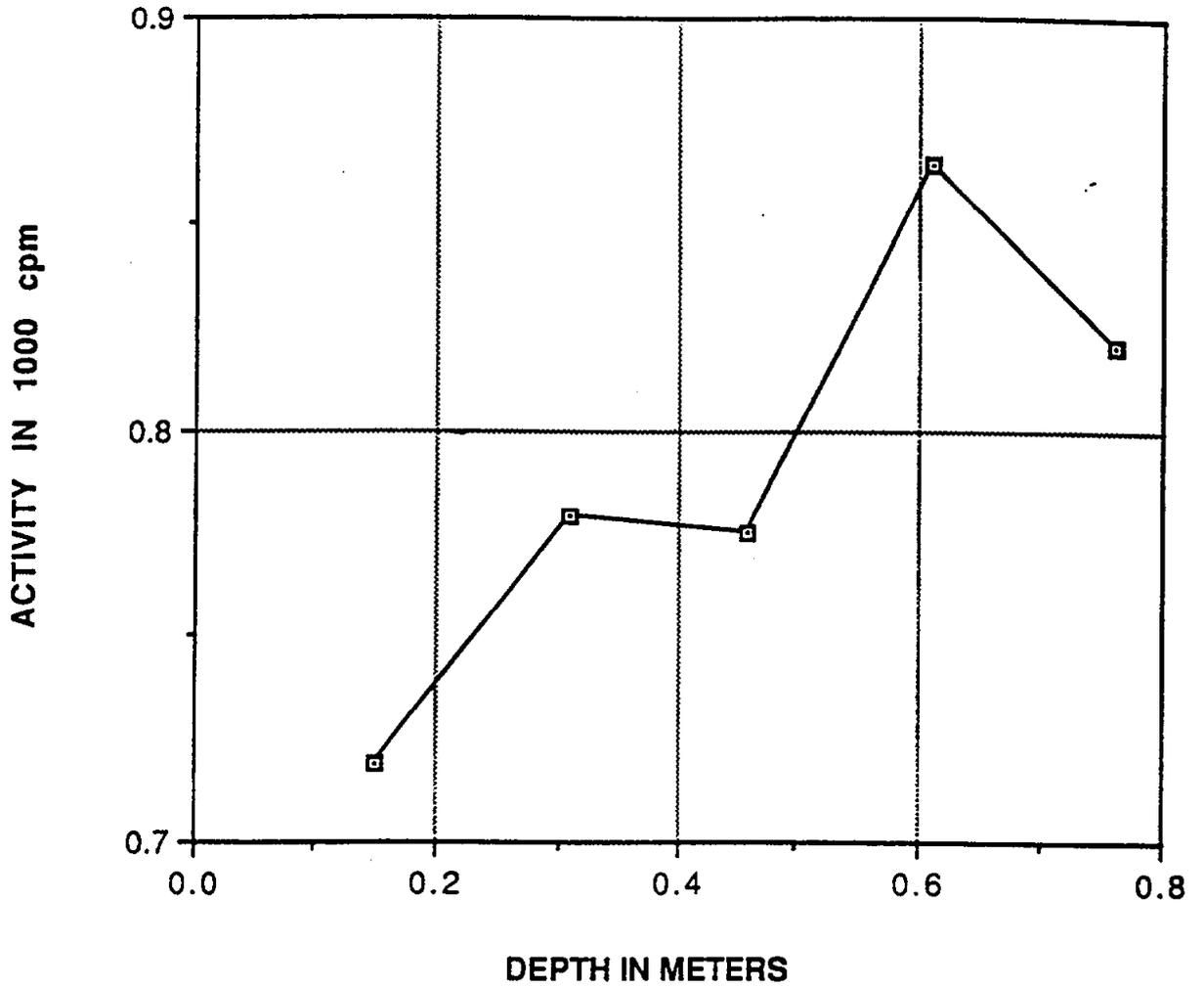
Fig. 3. Gamma profile for auger hole 2 (MJ041A2) at 142 West Central Avenue, Maywood, New Jersey.
