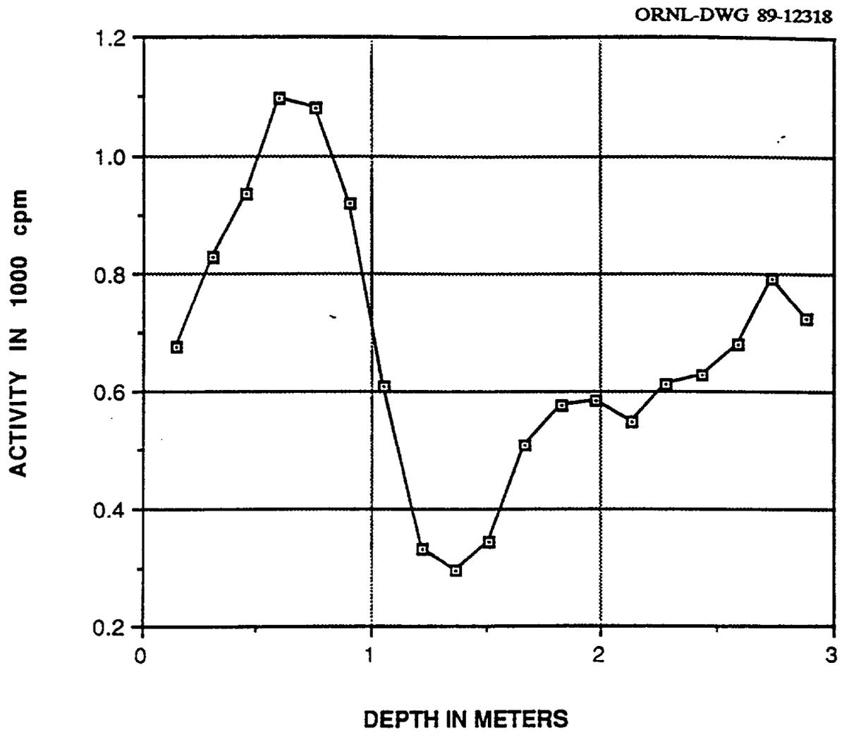
Fig. 4. Gamma profile for auger hole 3 (MJ041A3) at 142 West Central Avenue, Maywood, New Jersey.
