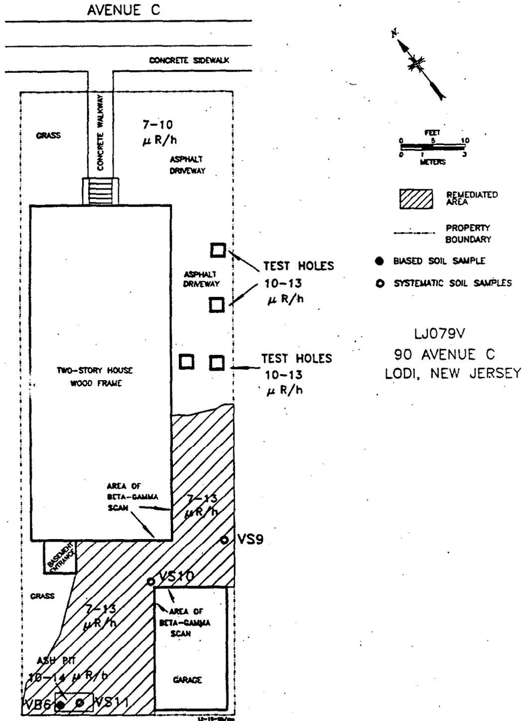
Fig. 2. Diagram of the property at 90 Avenue C, Lodi, New Jersey, showing surface gamma exposure rates and soil sampling locations.
