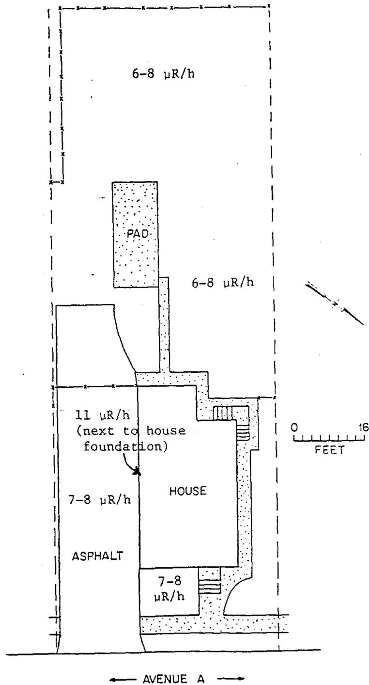
Fig. 2. Gamma radiation levels measured at 68 Avenue A, Lodi, New Jersey.
