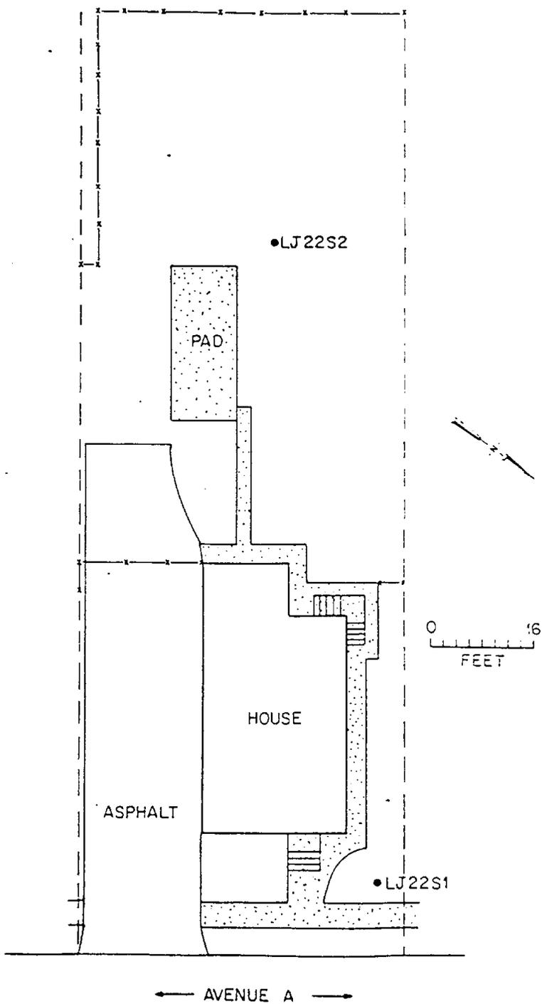
Fig. 1. Diagram showing locations of soil samples taken at 68 Avenue A, Lodi, New Jersey.
