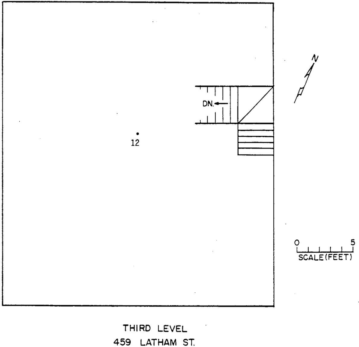
Fig. 8. Schematic of the third level floor plan at 459 Latham Street showing external gamma-ray measurement results at 1 m.
