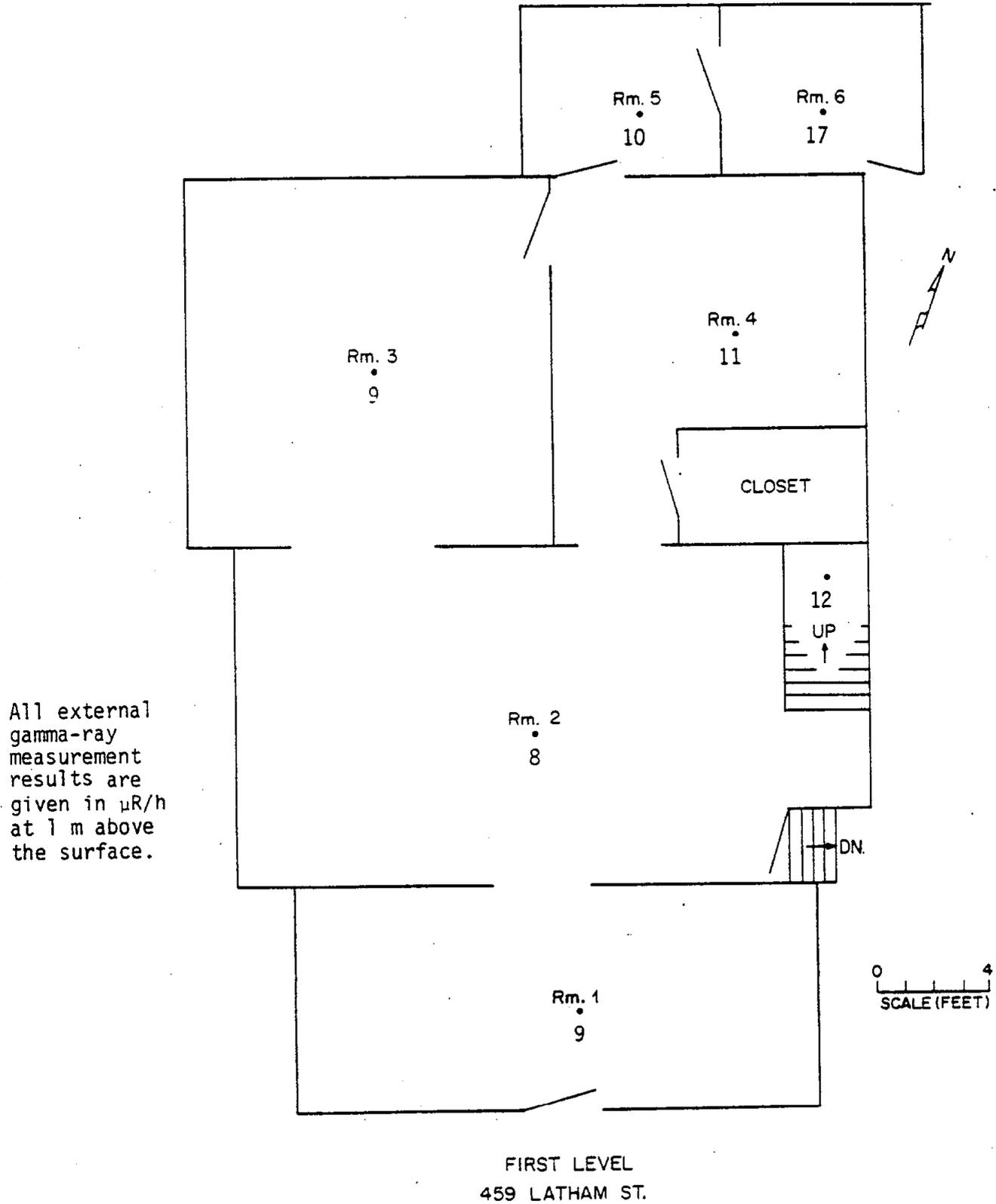
Fig. 6. Schematic of the first level floor plan at 459 Latham Street showing external gamma-ray measurement results at 1 m.
