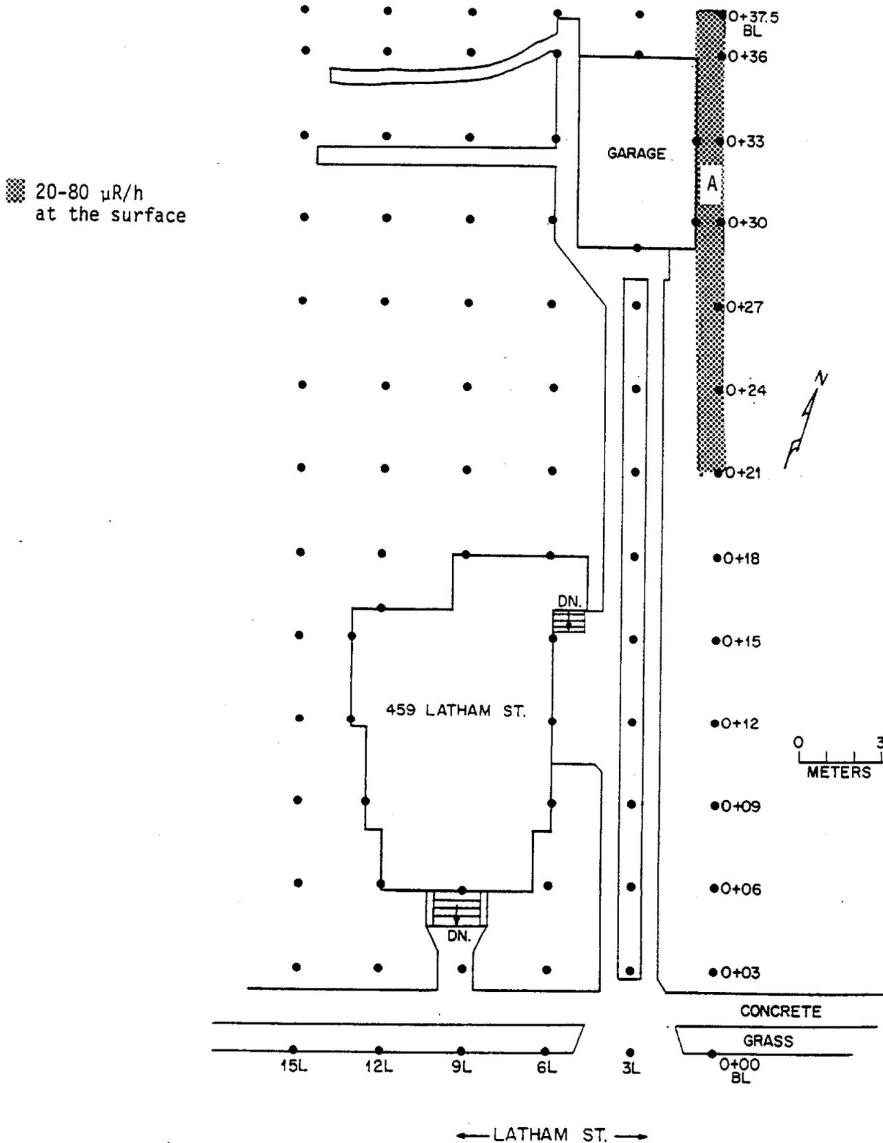
Fig. 4. Estimated extent of contaminated areas at 459 Latham Street based on results of external gamma-ray surface scan.
