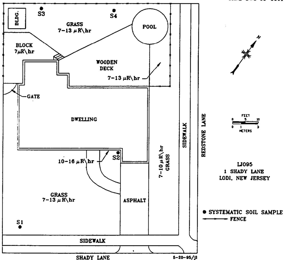
Fig. 2. Diagram showing gamma measurements and soil sampling locations at 1 Shady Lane, Lodi, New Jersey.
