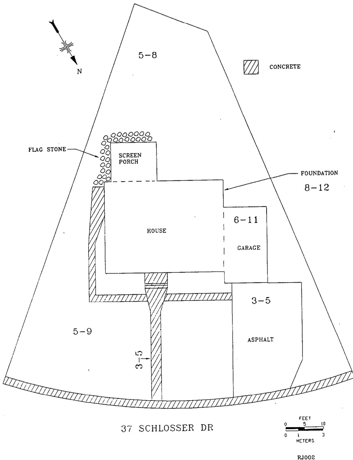
Fig. 1. Gamma radiation levels ( $\mu\text{R/h}$ ) measured on the surface at 37 Schlosser Drive, Rochelle Park, New Jersey (RJ002).
