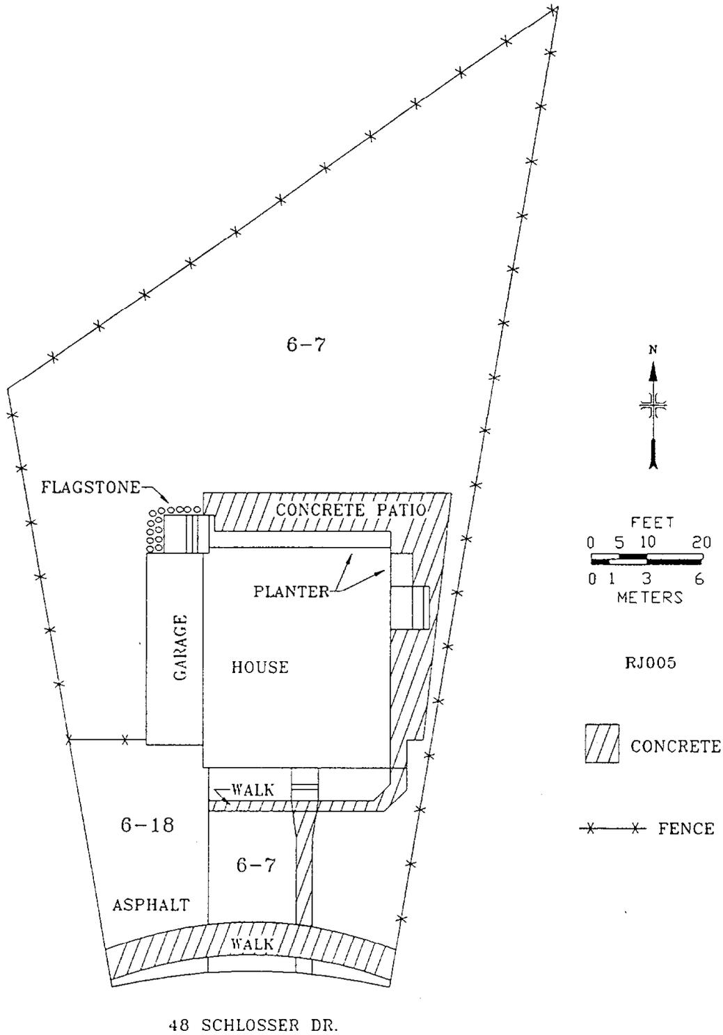
Fig. 1. Gamma radiation levels ( $\mu\text{R/h}$ ) measured on the surface at 48 Schlosser Drive, Rochelle Park, New Jersey (RJ005).
