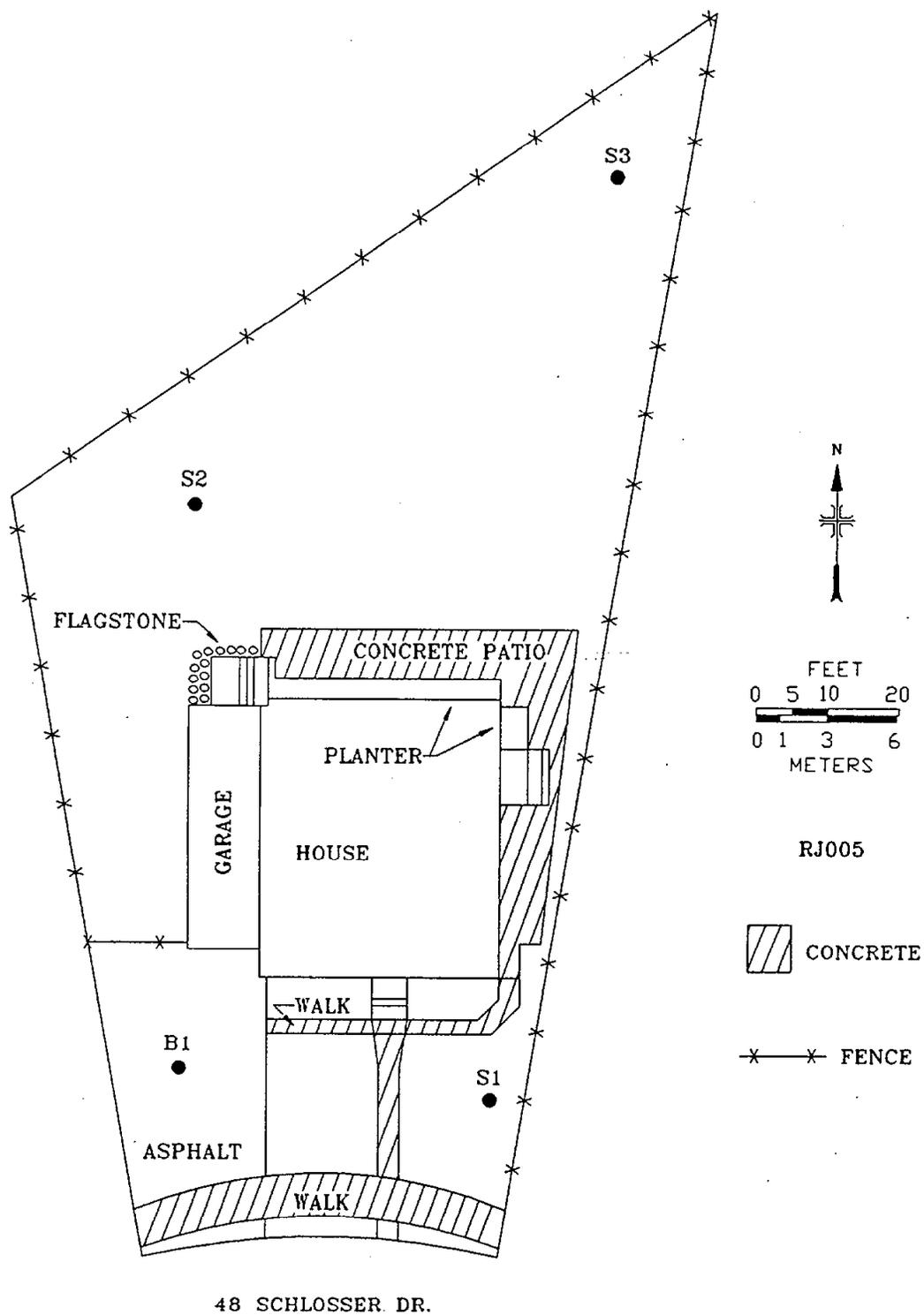
Fig. 2. Diagram showing locations of soil samples taken at 48 Schlosser Drive, Rochelle Park, New Jersey (RJ005).
