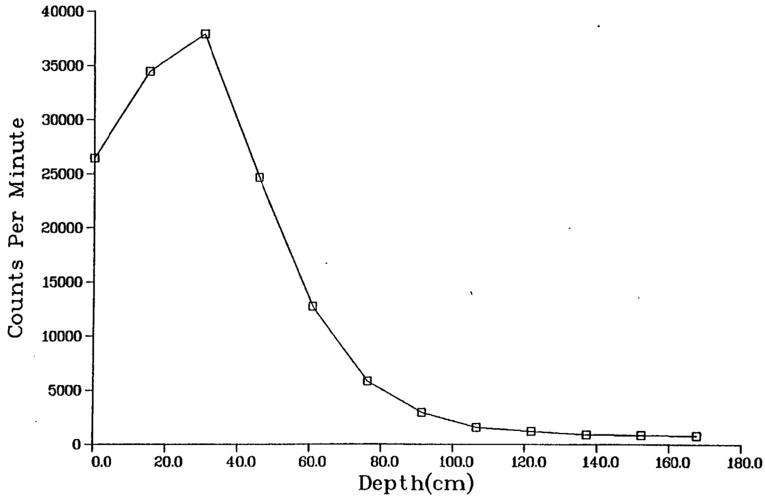
Fig. II-7. Gamma profile of core hole MJC25 (see Fig. 6)
