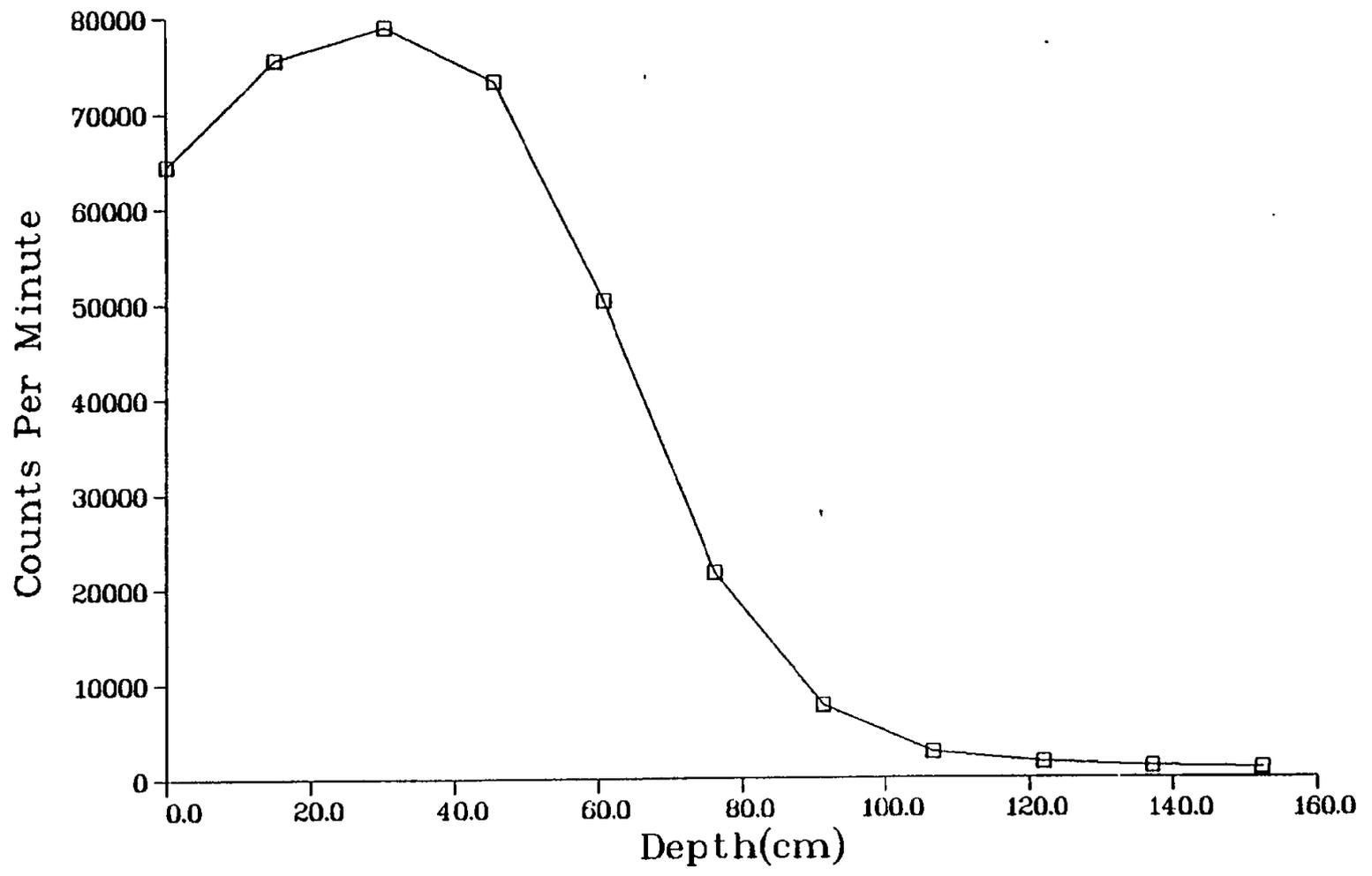
Fig. II-6. Gamma profile of core hole MJC24 (see Fig. 6)
