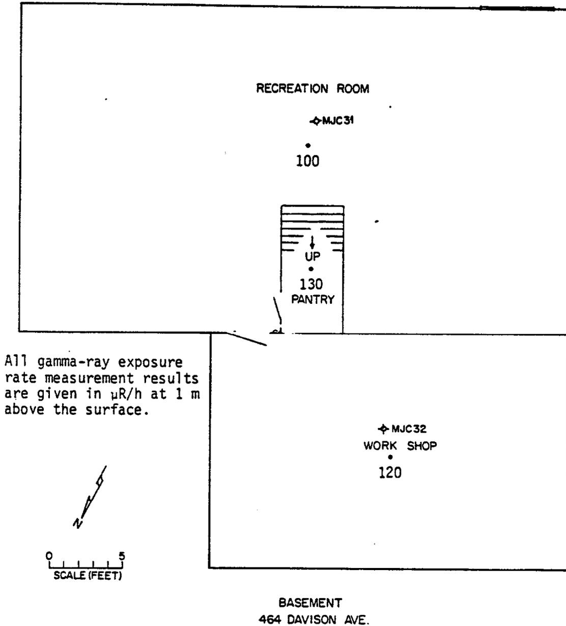
Fig. 8. Schematic of the basement floor plan at 464 Davison Avenue showing locations of drill holes and external gamma-ray measurement results.
