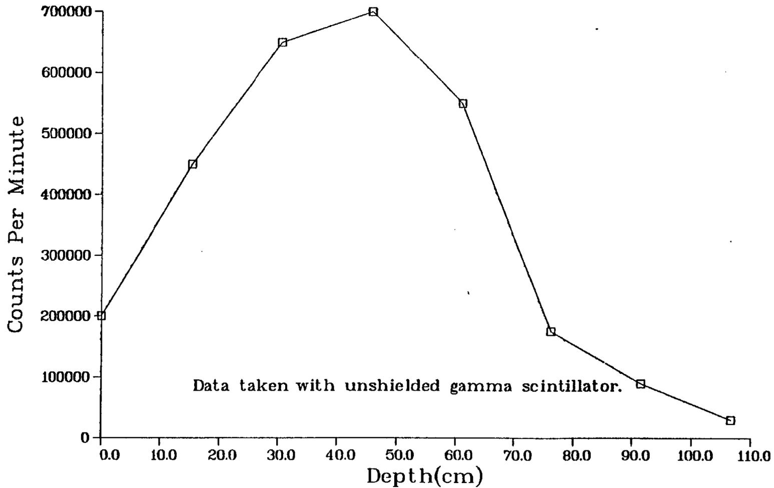
Fig. II-13. Gamma profile of core hole MJC31 (see Fig. 8)
