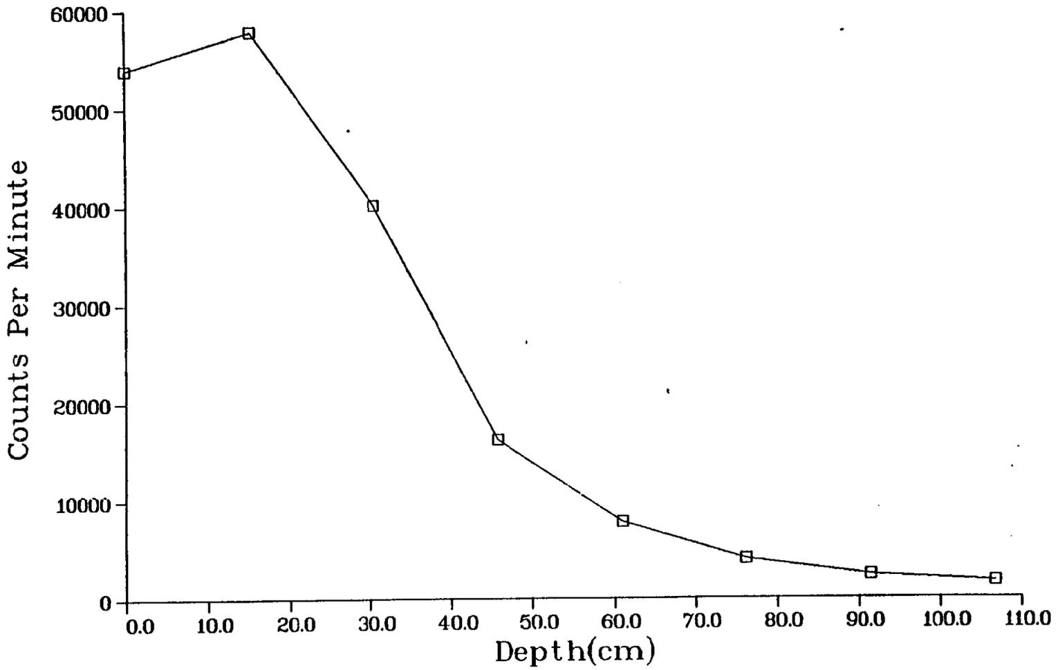
Fig. II-1. Gamma profile of core hole MJC19 (see Fig. 6)
