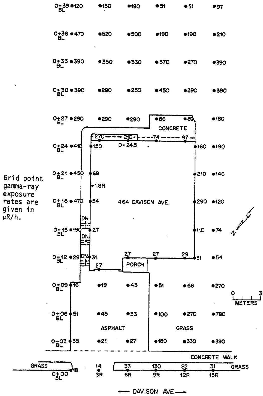
Fig. 4. External gamma-ray measurements at the ground surface at 464 Davison Avenue.
