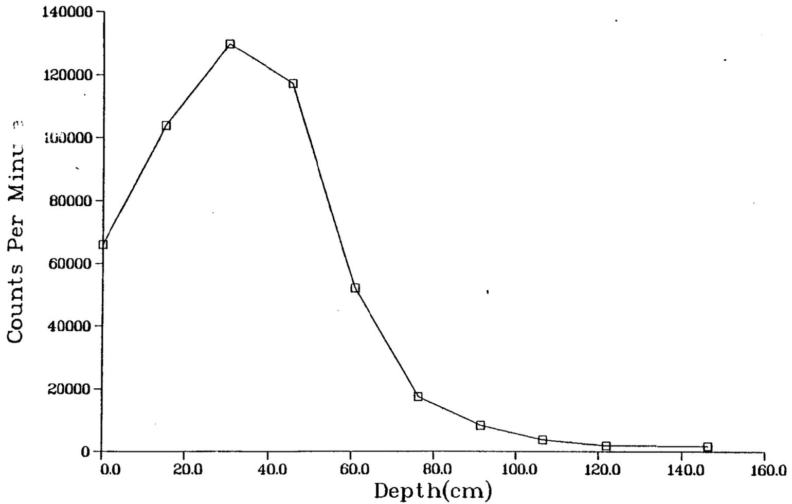
Fig. II-2. Gamma profile of core hole MJC20 (see Fig. 6)
