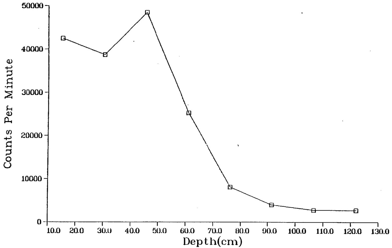
Fig. II-10. Gamma profile of core hole MJC28 (see Fig. 6)
