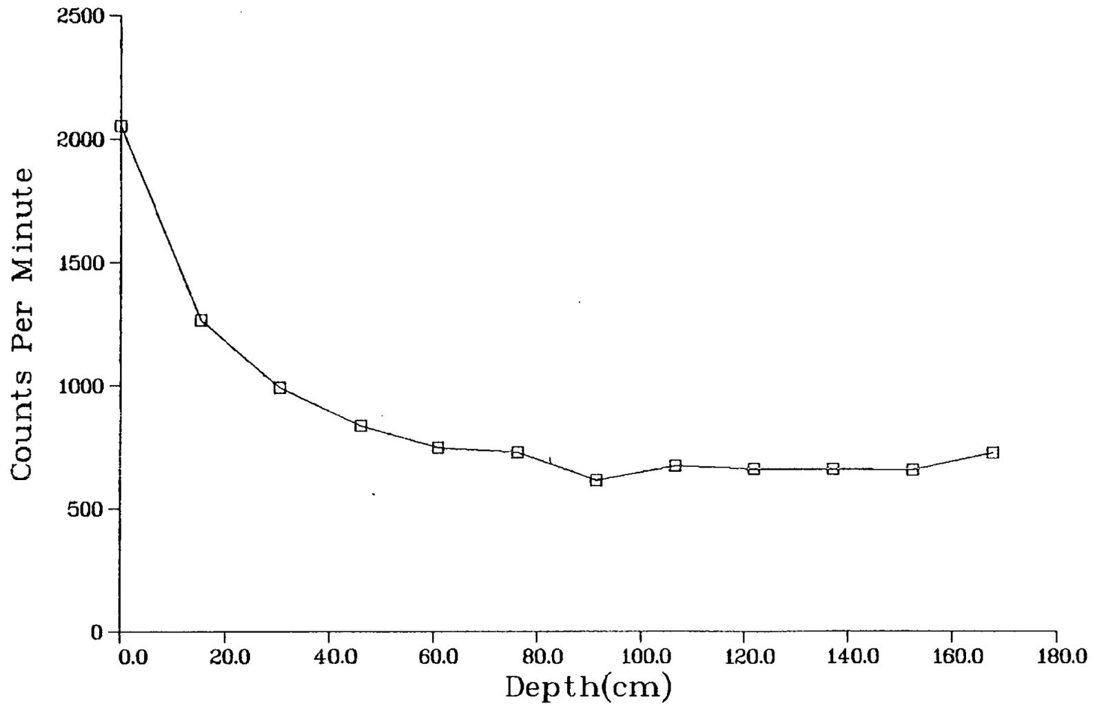
Fig. II-2. Gamma profile of core hole MJC40 (see Fig. 6)
