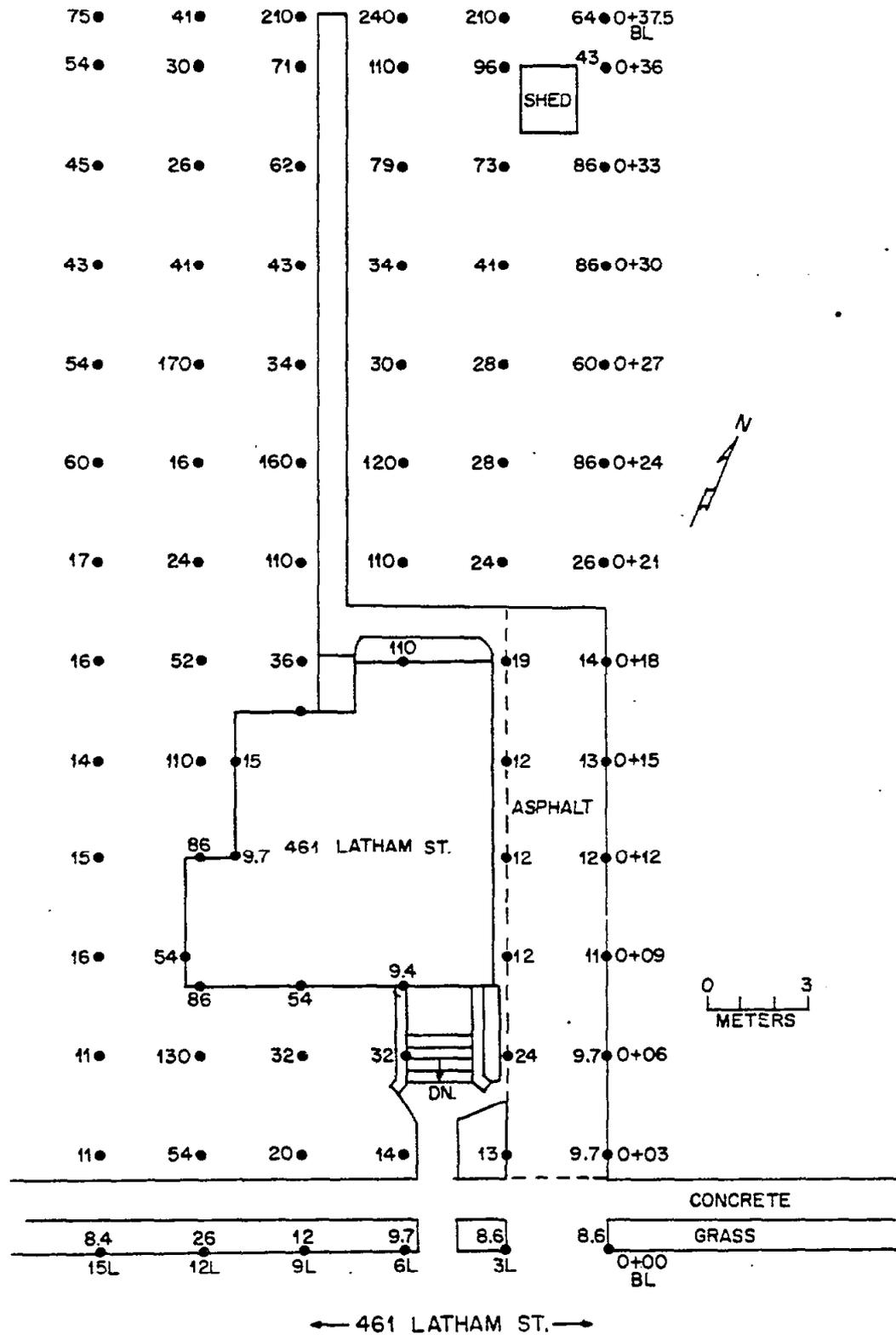
Fig. 4. Surface external gamma-ray exposure rates ( $\mu\text{R/h}$ ) at grid points at 461 Latham Street
