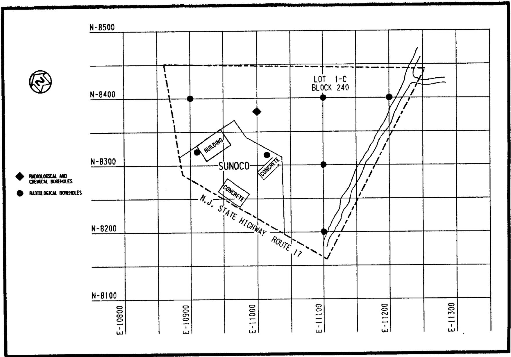
FIGURE 3-3 BOREHOLE LOCATIONS AT THE SUNOCO STATION PROPERTY
