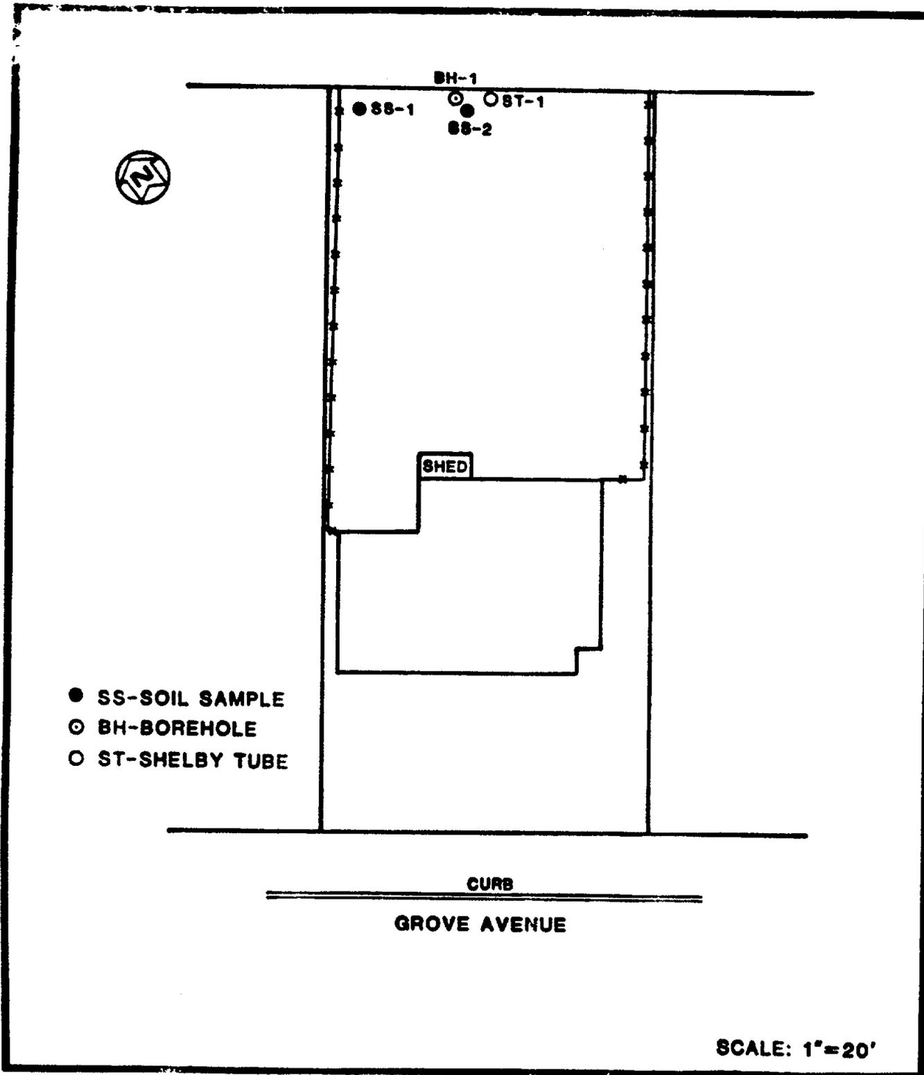
**FIGURE 3-1** LOCATIONS OF SURFACE SOIL SAMPLES, BOREHOLE, AND SHELBY TUBE CORE SAMPLE AT 46 GROVE AVENUE
