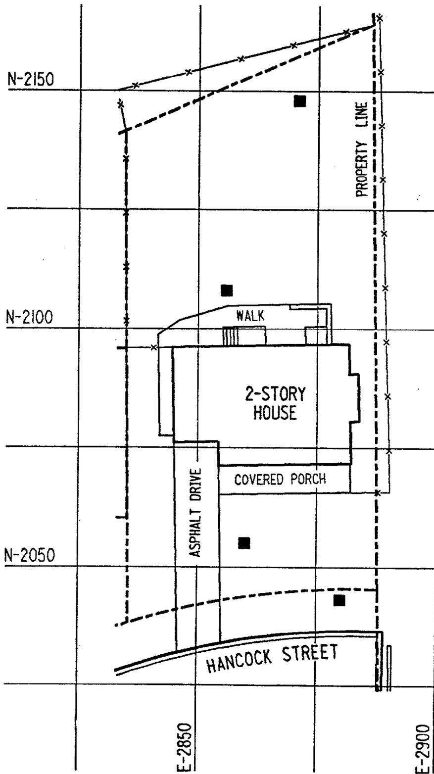
FIGURE 4-3 GAMMA EXPOSURE RATE MEASUREMENT LOCATIONS AT 9 HANCOCK STREET
