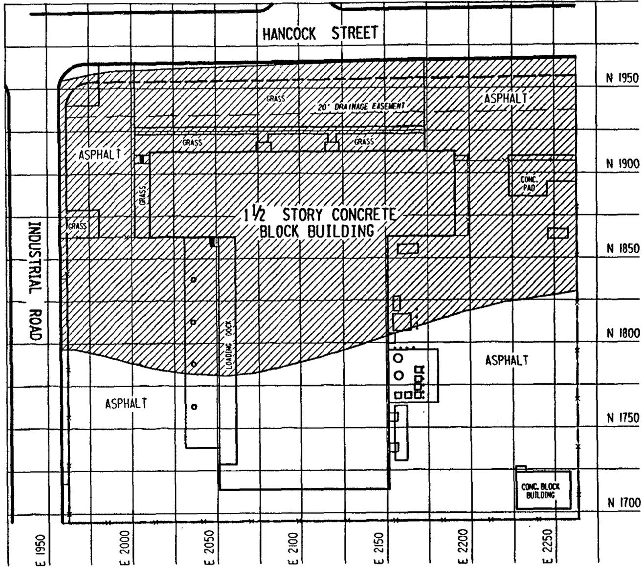
FIGURE 5-2 AREAS OF SUBSURFACE CONTAMINATION AT 80 HANCOCK STREET
