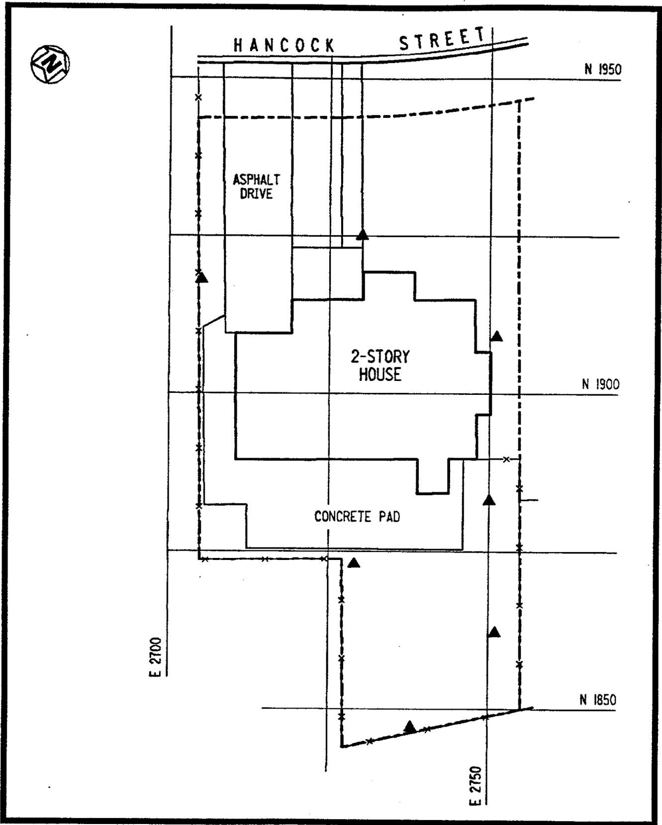
FIGURE 4-2 SURFACE AND SUBSURFACE SOIL SAMPLING LOCATIONS AT 4 HANCOCK STREET
