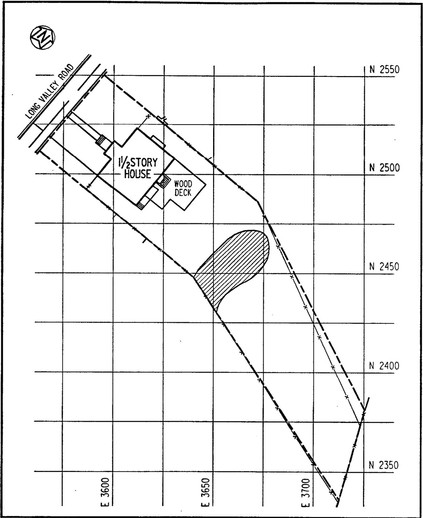
FIGURE 5-2 AREAS OF SUBSURFACE CONTAMINATION
