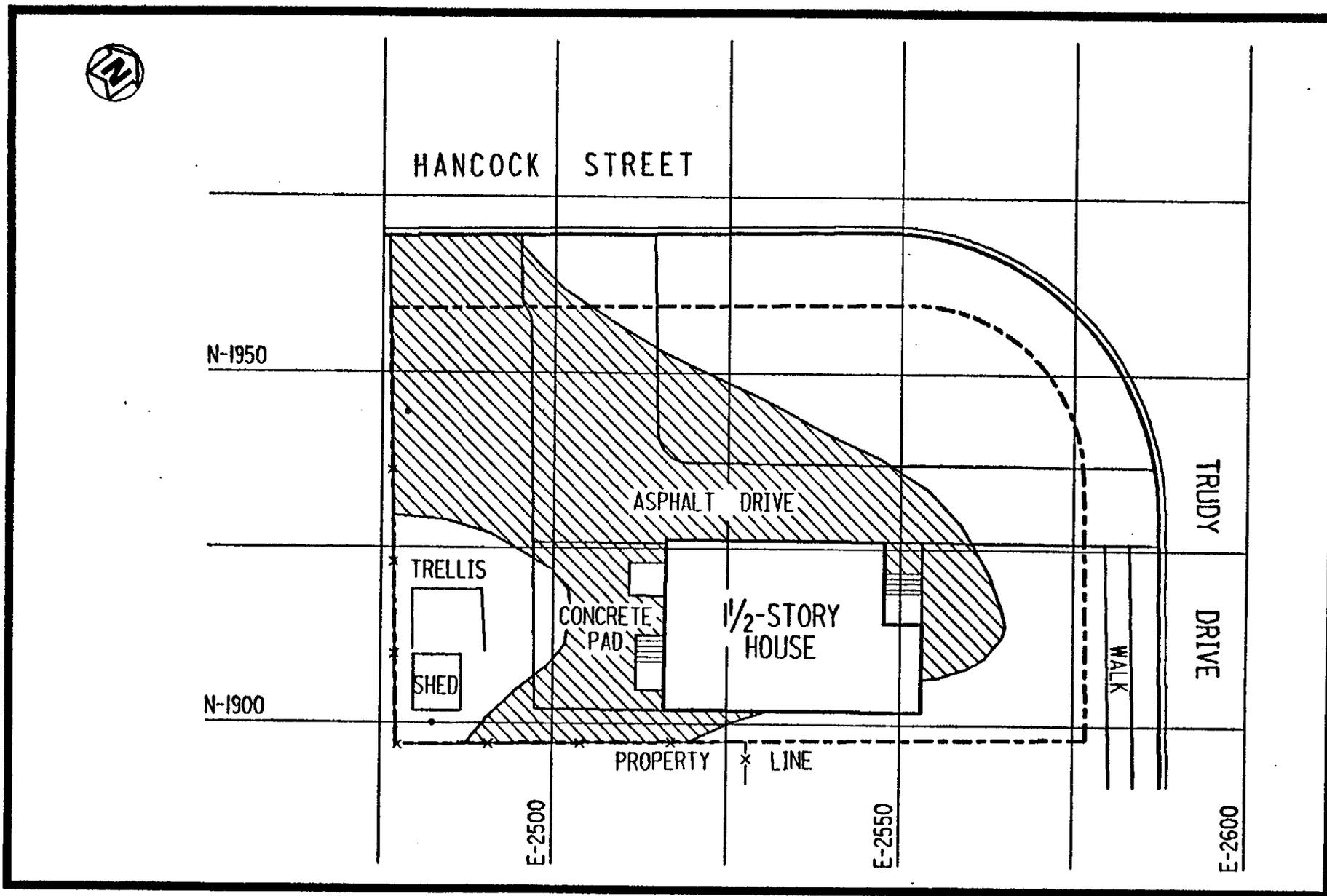
FIGURE 5-1 AREAS OF SURFACE CONTAMINATION AT 60 TRUDY DRIVE
