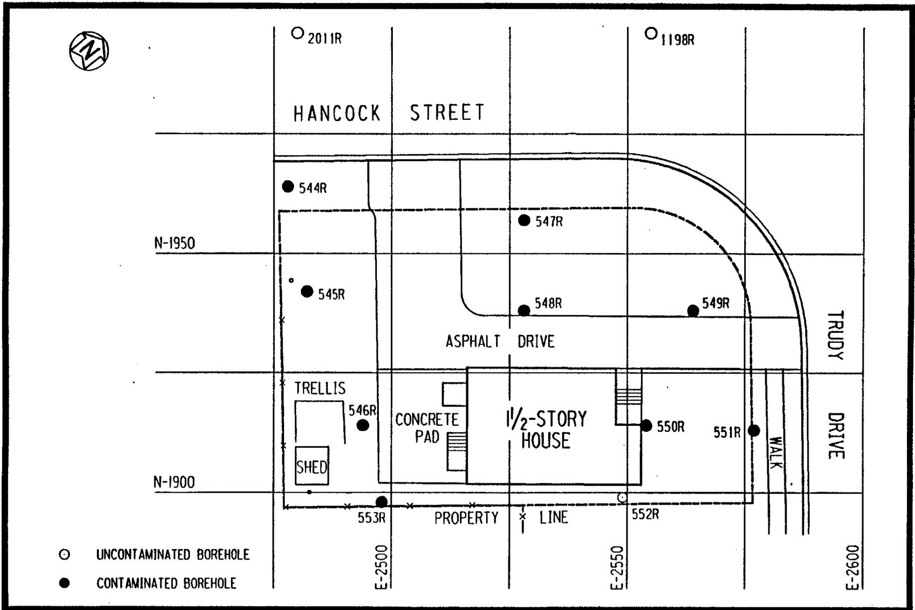
FIGURE 4-1 BOREHOLE LOCATIONS AT 60 TRUDY DRIVE
