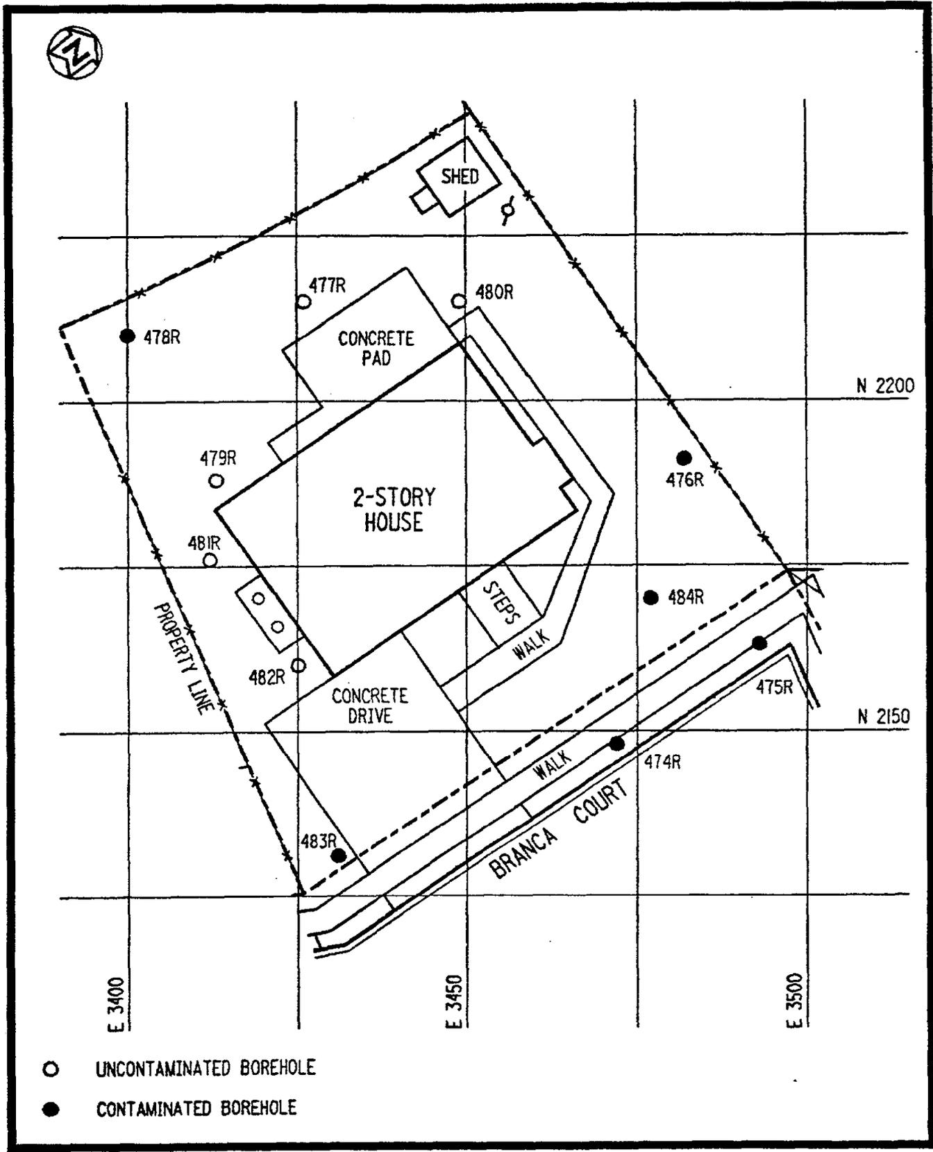
FIGURE 4-1 BOREHOLE LOCATIONS AT 6 BRANCA COURT
