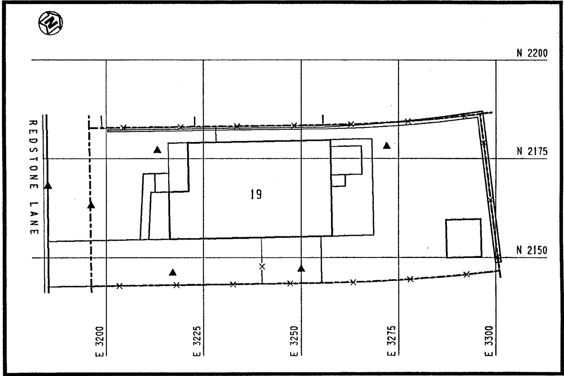
FIGURE 4-2 SURFACE AND SUBSURFACE SOIL SAMPLING LOCATIONS AT 19 REDSTONE LANE
