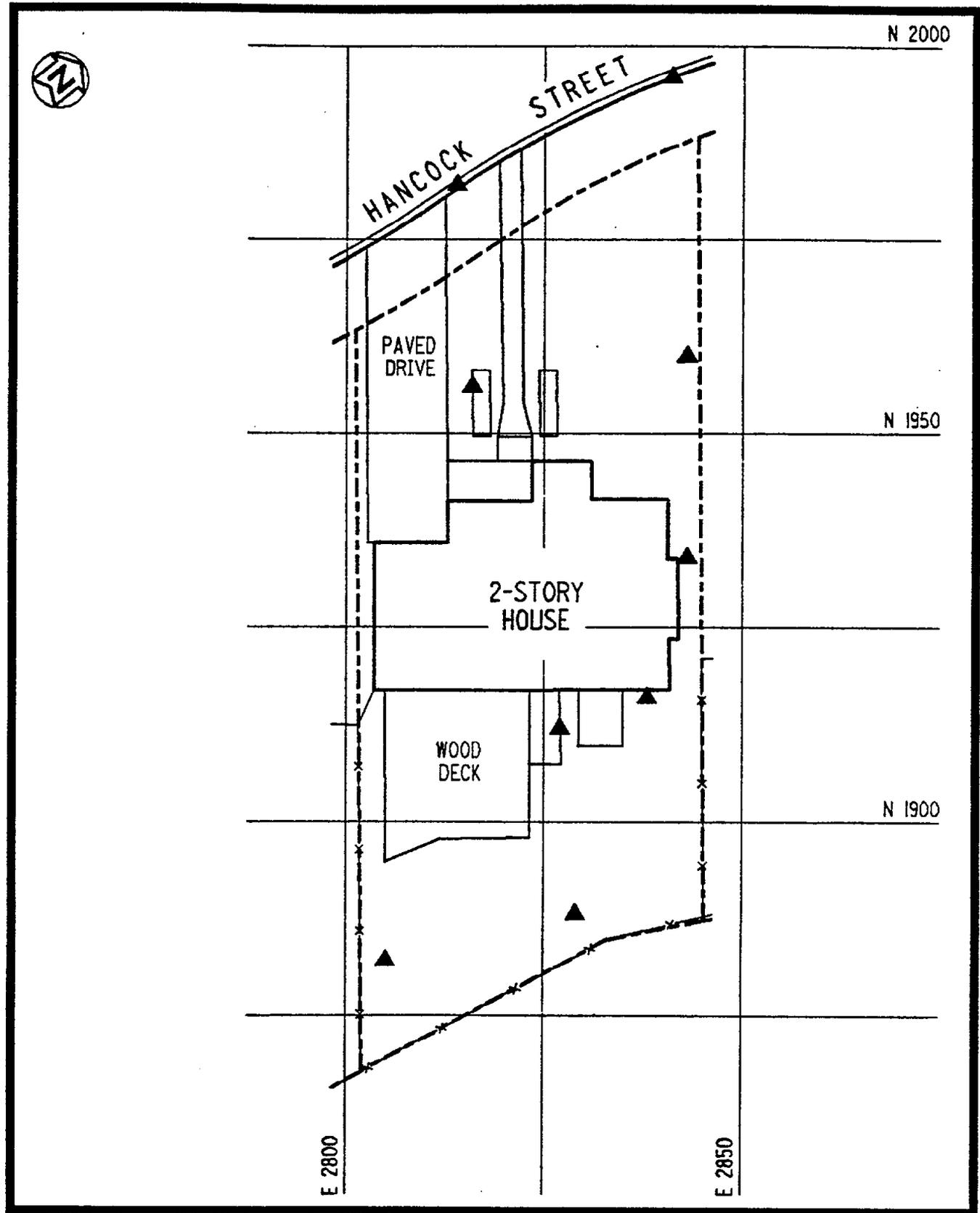
FIGURE 4-2 SURFACE AND SUBSURFACE SOIL SAMPLING LOCATIONS AT 8 HANCOCK STREET
