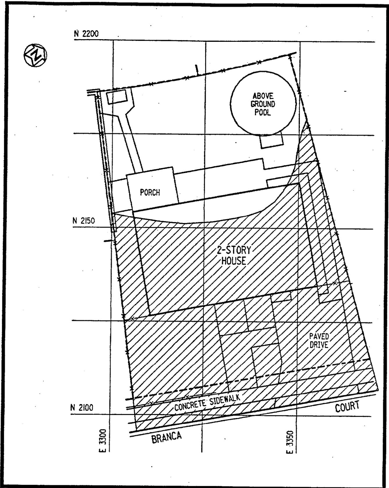
FIGURE 5-1 AREAS OF SUBSURFACE CONTAMINATION AT 2 BRANCA COURT
