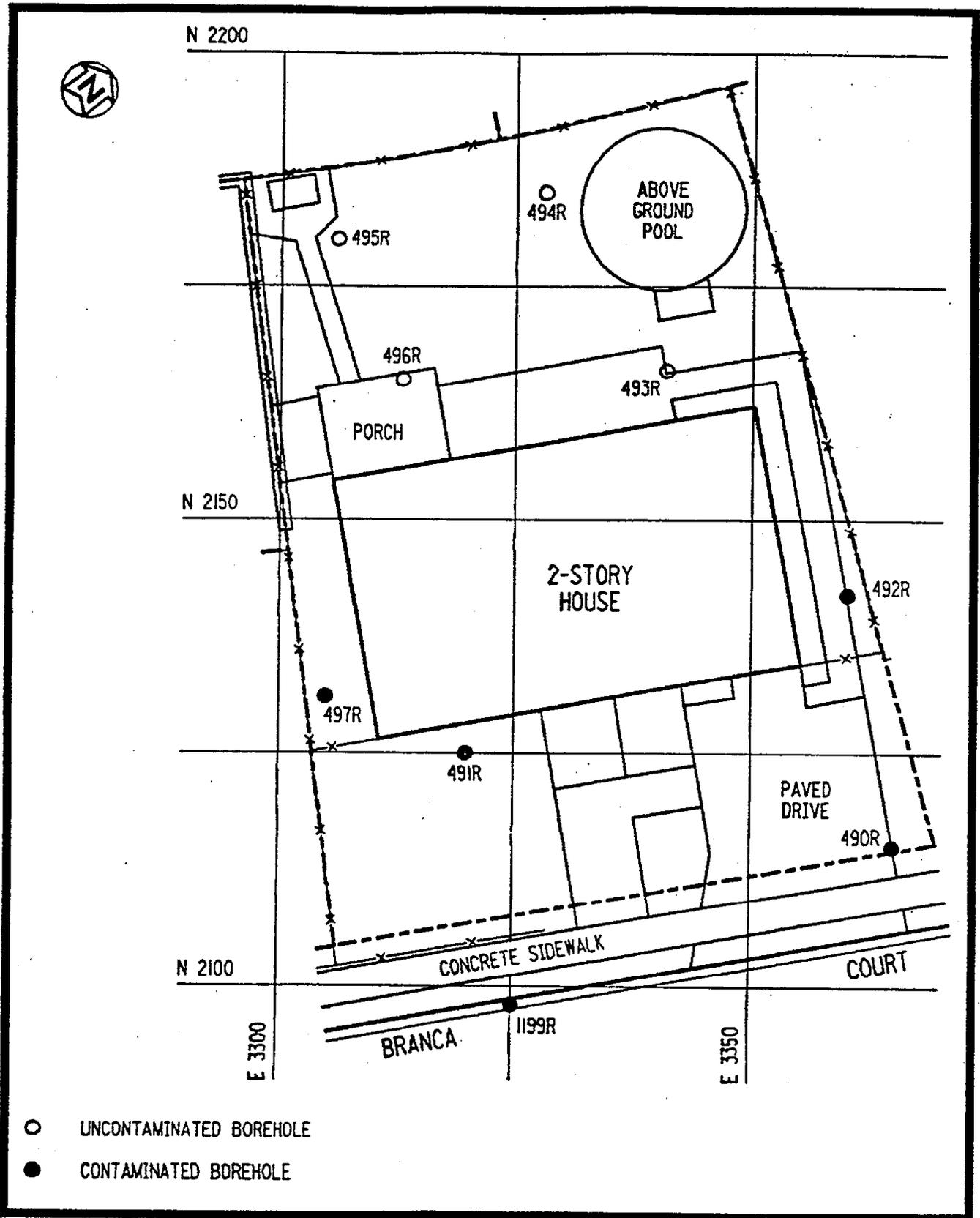
FIGURE 4-1 BOREHOLE LOCATIONS AT 2 BRANCA COURT
