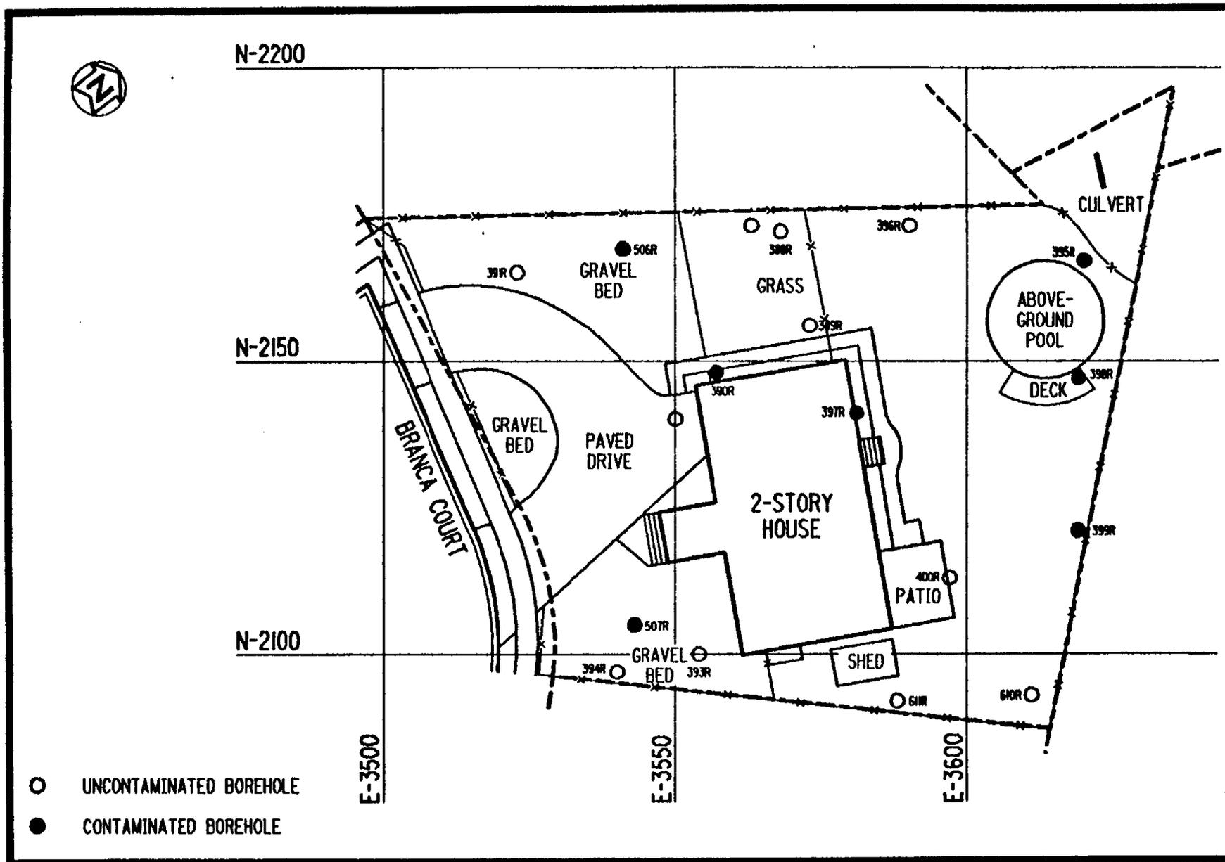
FIGURE 4-1 BOREHOLE LOCATIONS AT 11 BRANCA COURT
