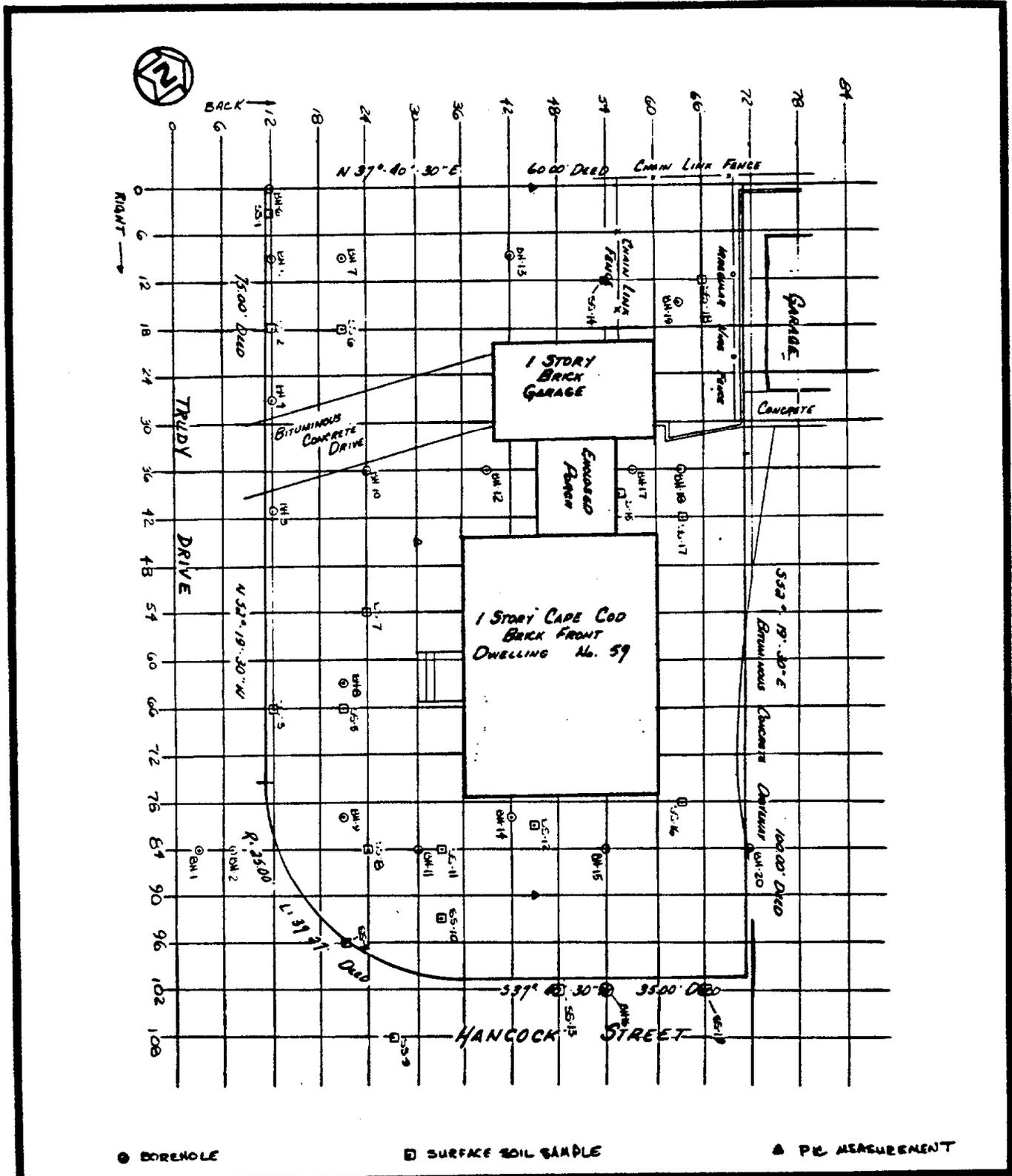
FIGURE 1 LOCATIONS OF BOREHOLES, SOIL SAMPLES, AND PIC MEASUREMENTS AT 59 TRUDY DRIVE
