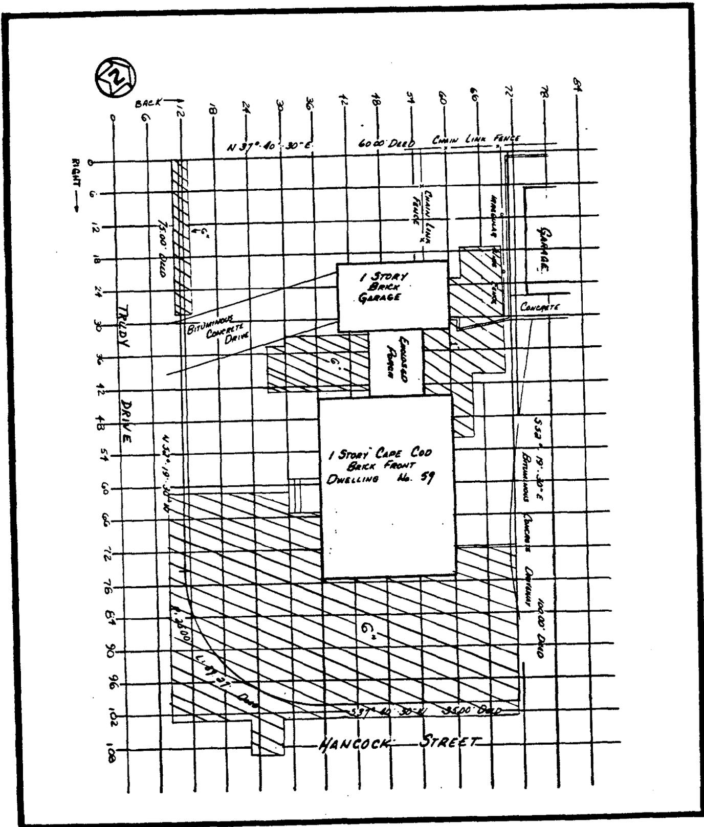
FIGURE 2 LOCATION OF ELEVATED GAMMA RADIATION LEVELS AT 59 TRUDY DRIVE
