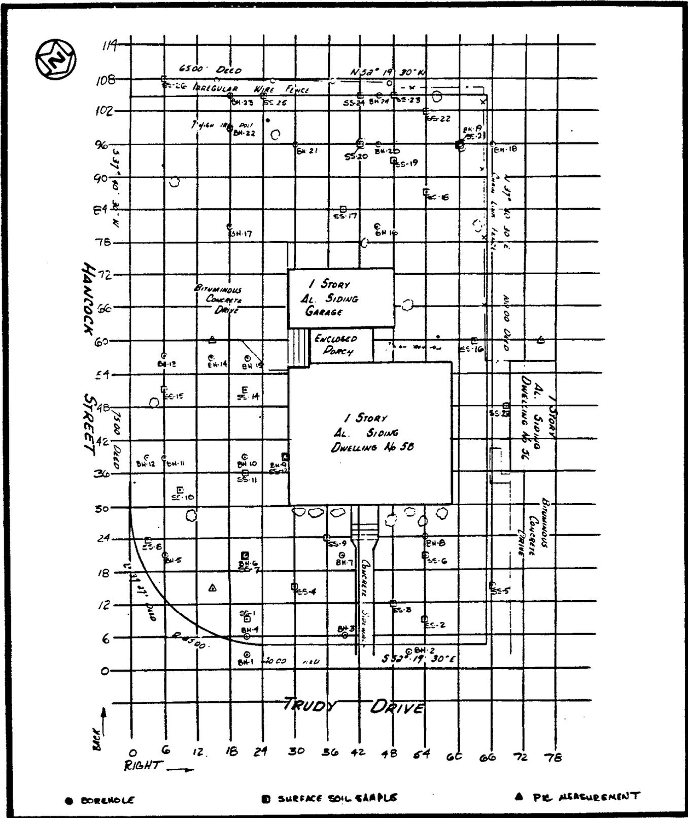
FIGURE 1 LOCATIONS OF BOREHOLES, SOIL SAMPLES, AND PIC MEASUREMENTS AT 58 TRUDY DRIVE
