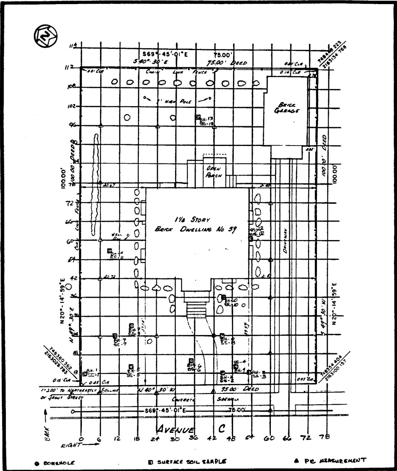
FIGURE 1 LOCATIONS OF BOREHOLES, SOIL SAMPLES, AND PIC MEASUREMENTS AT 59 AVENUE C
