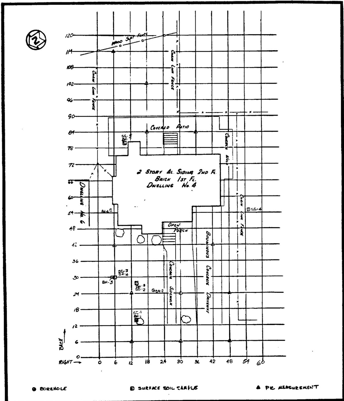
FIGURE 1 LOCATIONS OF BOREHOLES, SOIL SAMPLES, AND PIC MEASUREMENTS AT 4 HANCOCK STREET
