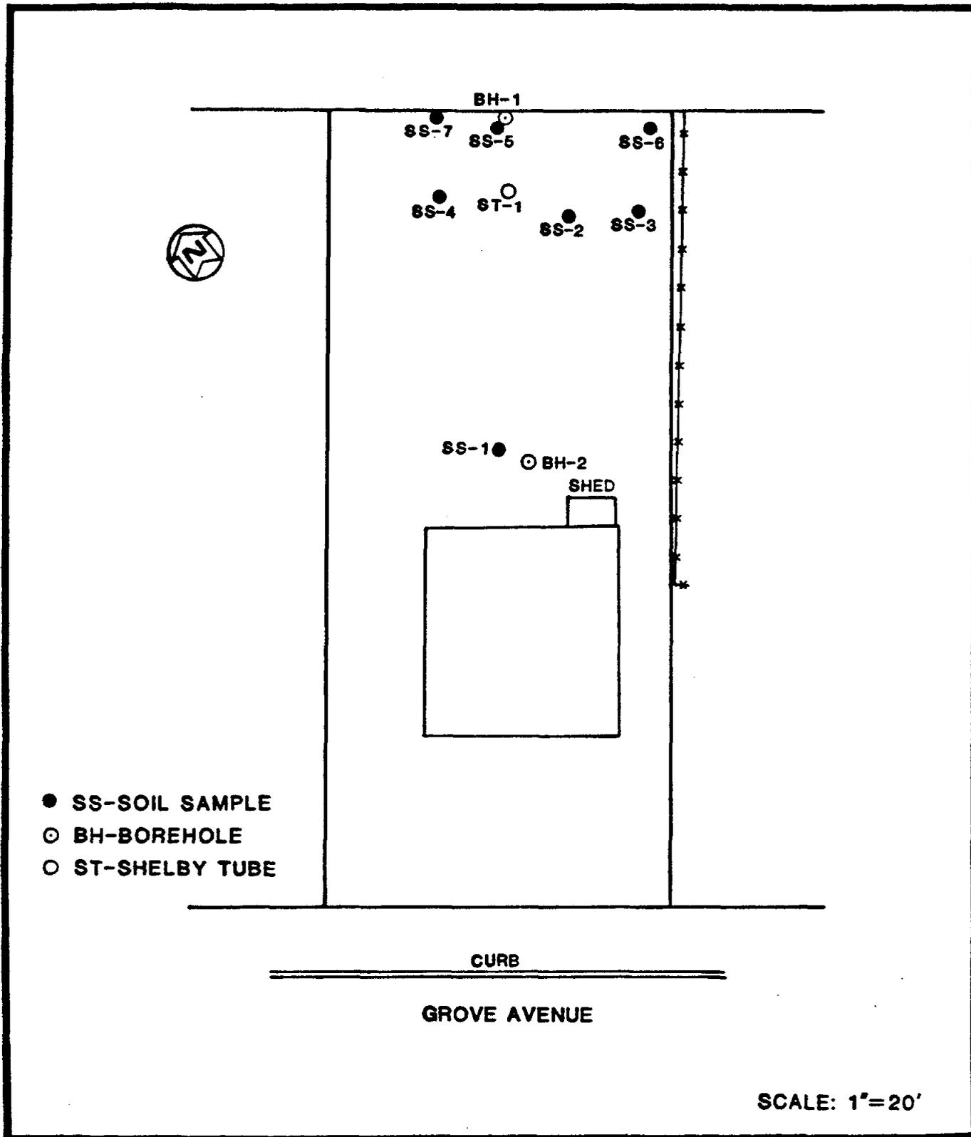
FIGURE 3-2 LOCATIONS OF SURFACE SOIL SAMPLES, BOREHOLES, AND SHELBY TUBE CORE SAMPLE AT 42 GROVE AVENUE
